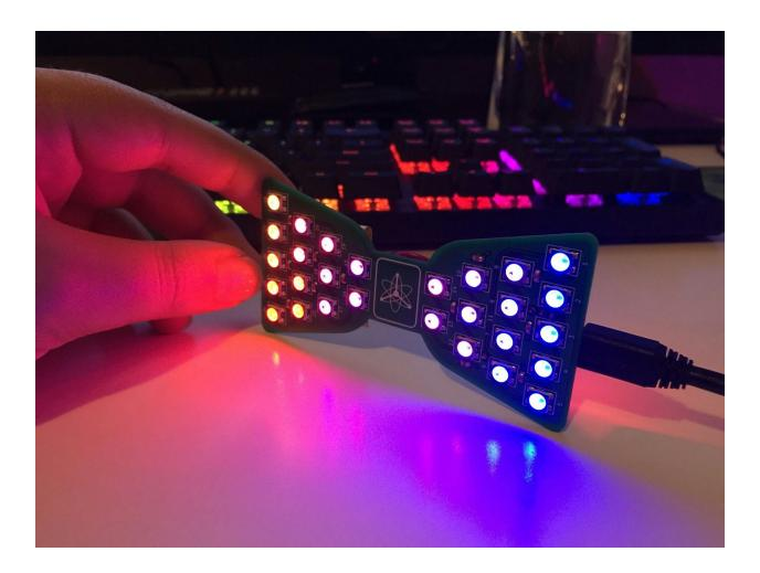
6. You're done! All that's left to do is tie the bow tie strap around the center of the Tinker Tie board (we like to also make sure it covers the battery wire) adjust it to your neck size and wear it! The Tinker Tie can be charged over USB, as well as programmed to your own custom patterns through the Arduino IDE. Enjoy your new Tinker Tie and please don't forget to send us any feedback you have of the process so we can further improve it beyond Beta!
