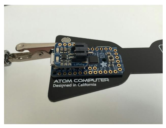
f. Once you're finished soldering, your Tinker Tie should look something like the image below from the side. Notice that the Pro Trinket is mounted at an angle, with the side with no pins to solder resting on the Tinker Tie board. This is the correct configuration.
