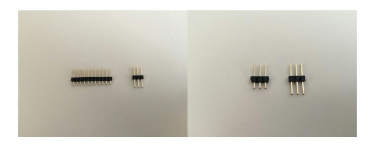
c. Next, Place the headers block with the longer pins into the first set of holes, followed by the shorter one.
