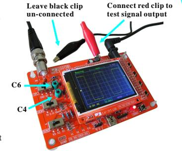
1. Connect the red clip to the test signal terminal and leave the black clip un-connected (see photo at right).
