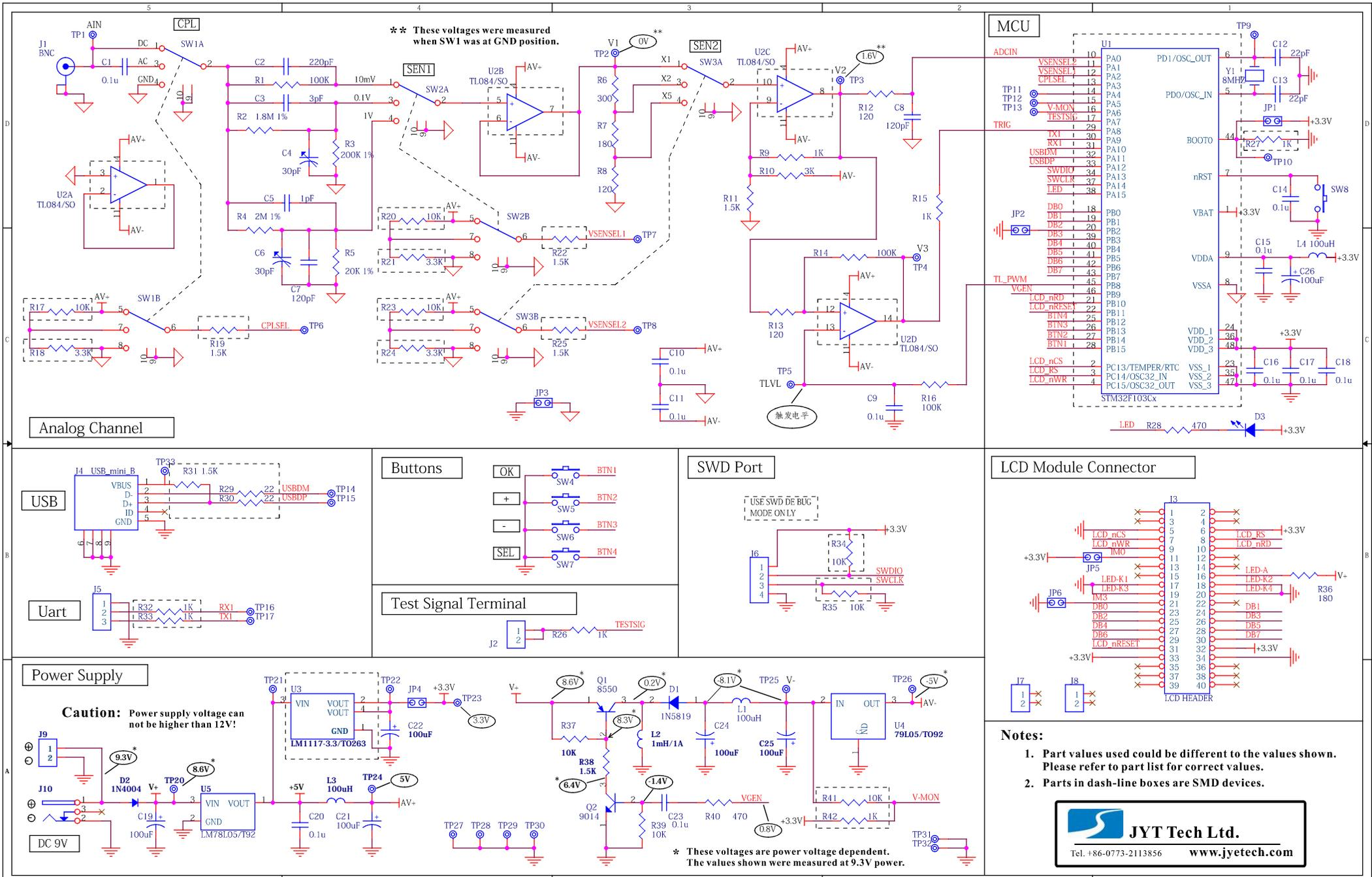
\*\* These voltages were measured when SW1 was at GND position.
