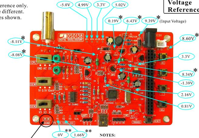
Place the negative pen of volt-meter here to do voltage measurements.
