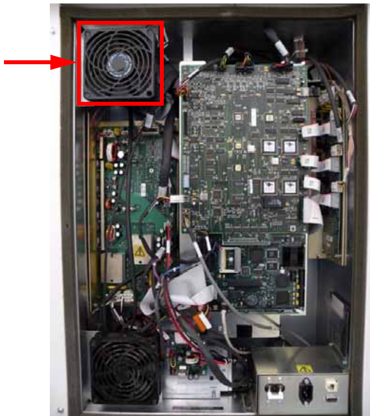
Figure 173: Dual 48 VDC power supply location
