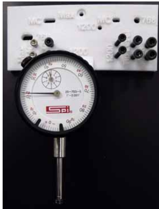
Figure 25: Dial indicator installation
