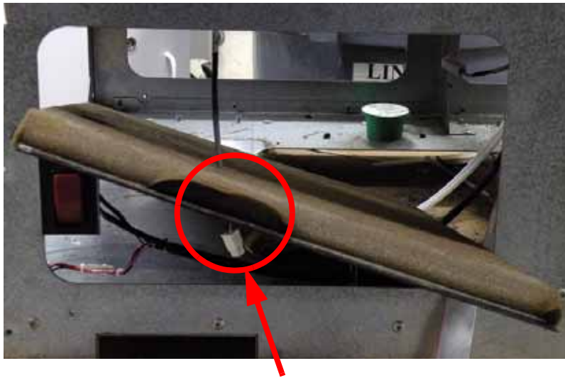
Figure 500: Z stage base plate removal
