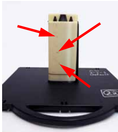
Example of embedded support
