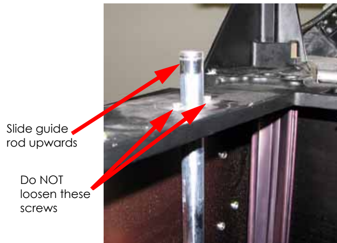
Figure 523: Removing the guide rods
