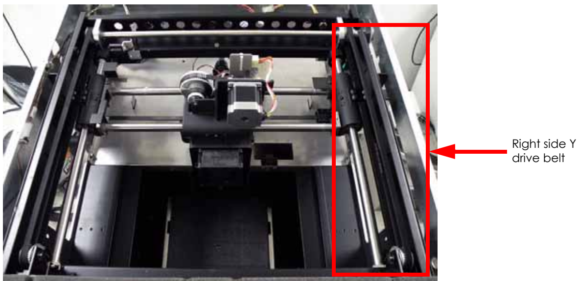
Figure 350: Right side Y drive belt location
