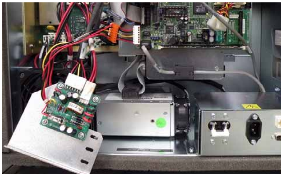
Figure 188: Setting the 5 VDC piggyback power supply off to the side
