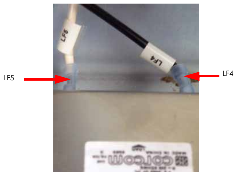
Figure 199: Line filter rear connection locations
