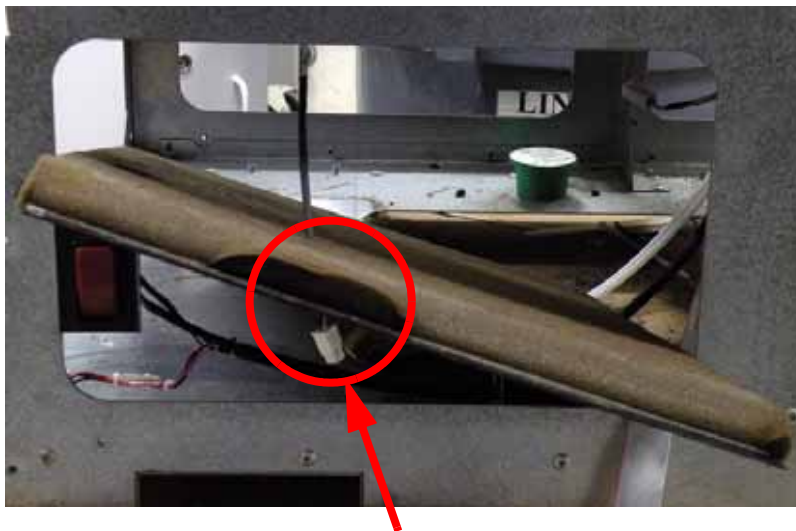
Figure 514: Z stage base plate removal
