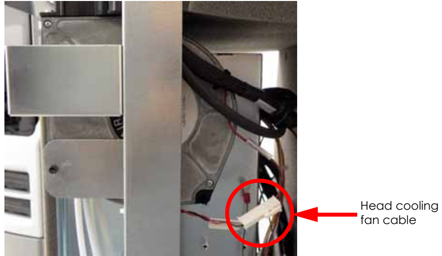
Figure 211: Fan cable location
