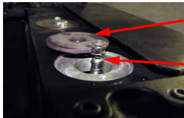
Figure 520: Removing the bearing caps and springs
