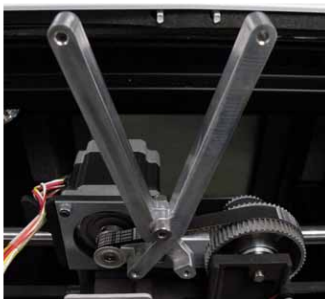
Figure 35: XY belt tension tool placement
