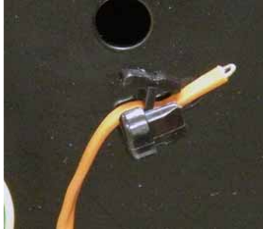
Figure 544: Removing the chamber thermocouple
