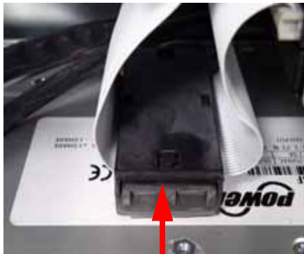
Figure 158: Ribbon cable ferrite location
