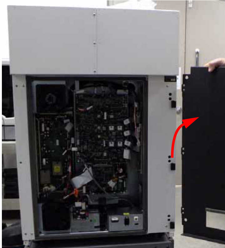
Figure 2: Removing rear door
