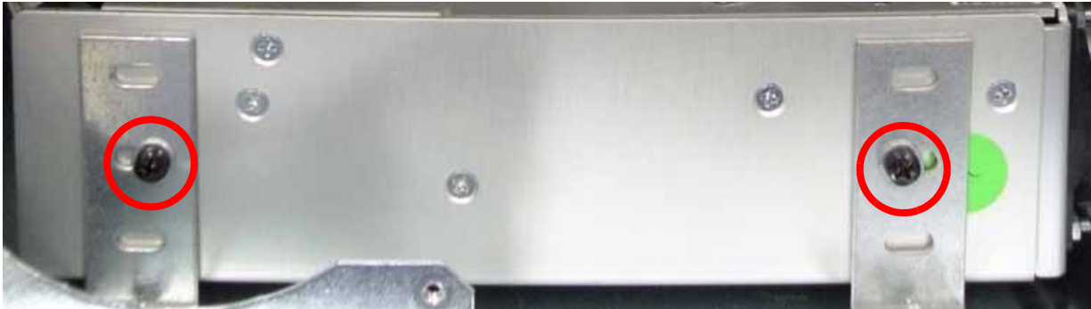
Figure 167: L bracket mounting screw locations
