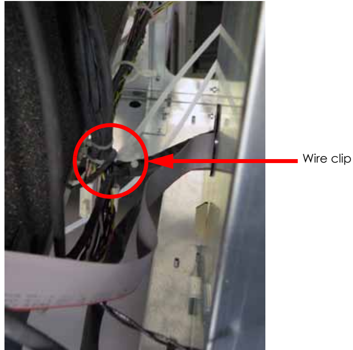
Figure 564: Z jam sensor wire clip location
