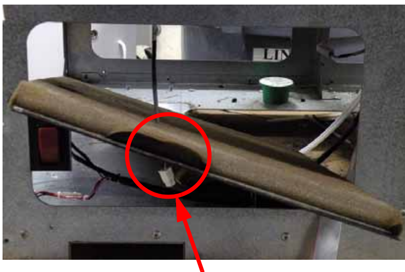
Figure 482: Z stage base plate removal
