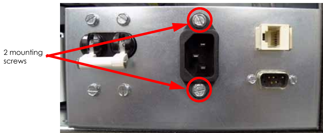
Figure 203: AC input mounting screw locations
