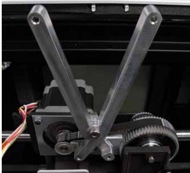
Figure 317: XY belt tension tool placement
