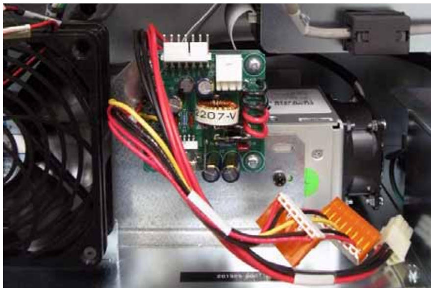
Figure 148: 5 VDC piggyback supply and mounting bracket
