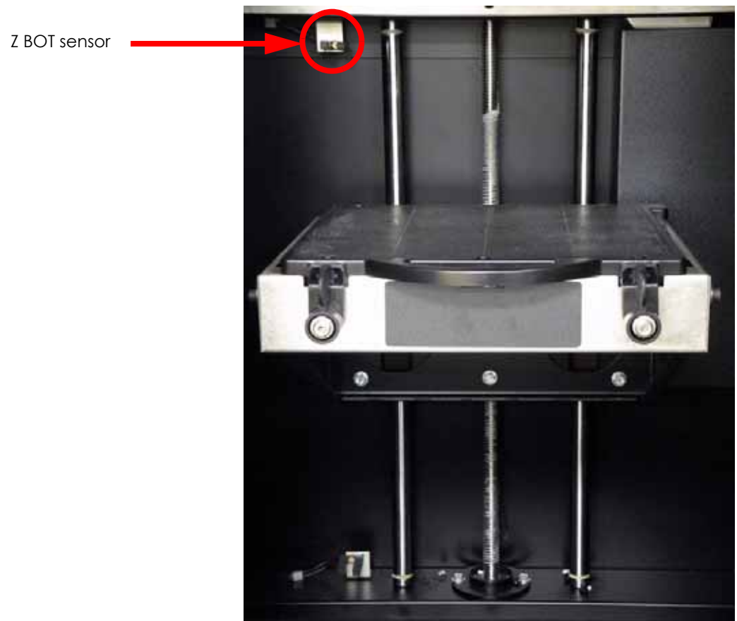
Figure 567: Z BOT sensor location
