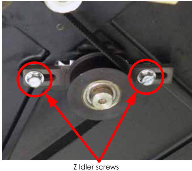
Figure 502: Z motor belt tension idler pulley screw locations
