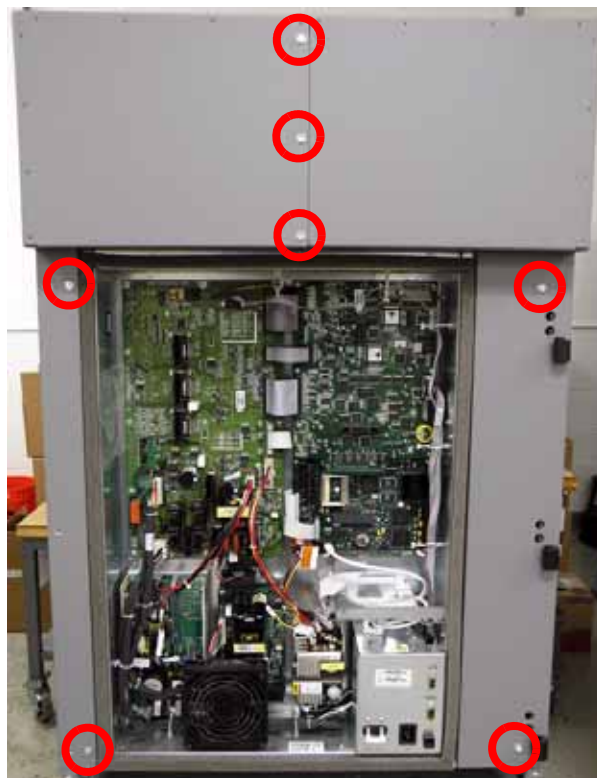
Figure 4: Side panel mounting screw locations
