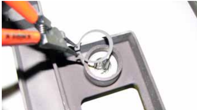
Figure 525: Bearing retaining clip
