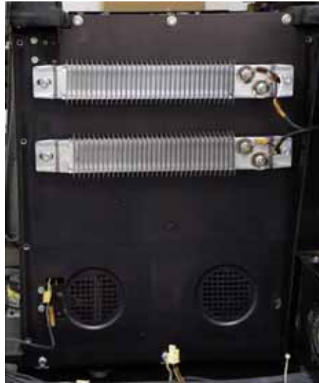
Figure 63: Opening the chamber heater cover
