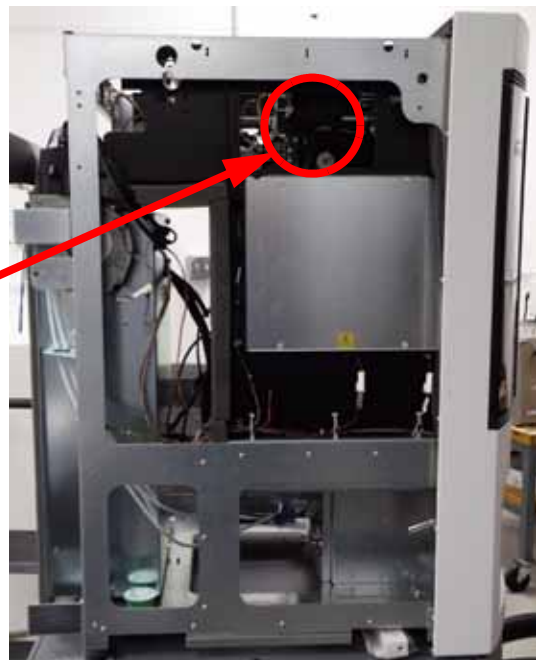
Figure 332: Left side X drive belt clamp location
