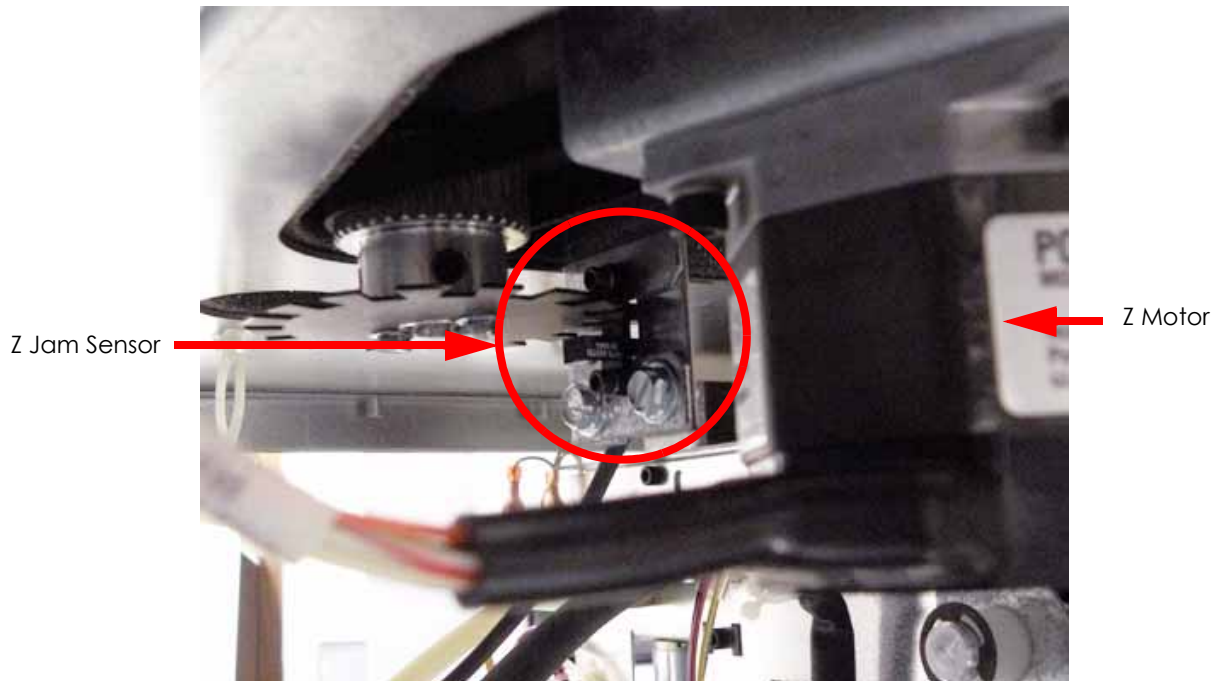
Figure 583: Z jam sensor location
