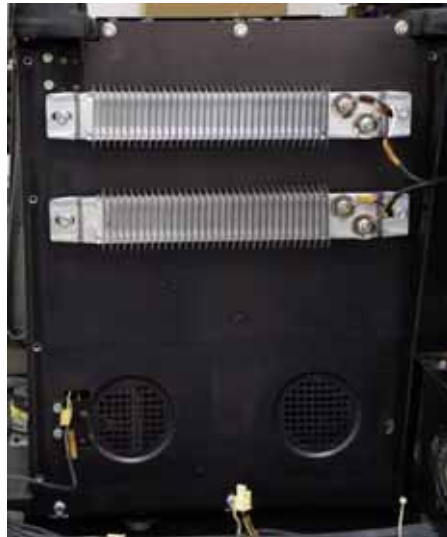
Figure 474: Opening the chamber heater cover
