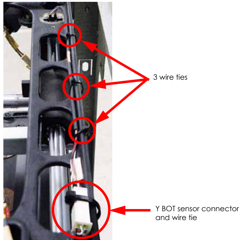
Figure 281: Wire tie and Y BOT connector locations
