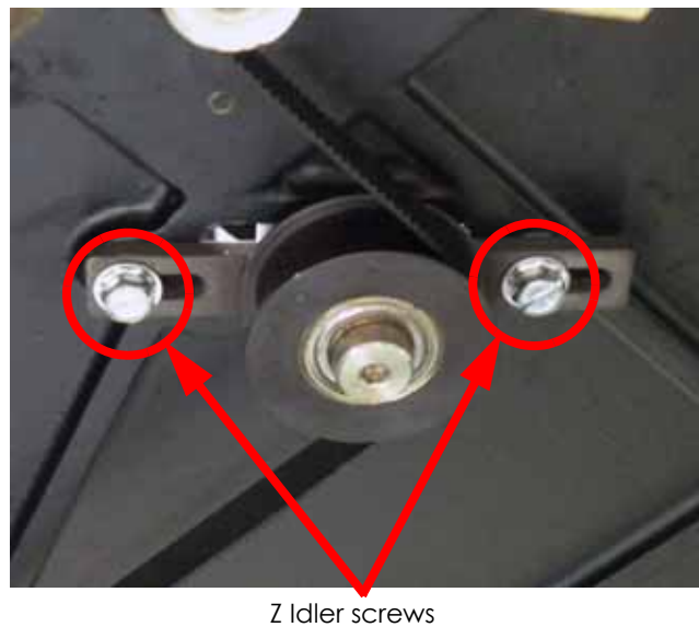
Figure 516: Z motor belt tension idler pulley screw locations
