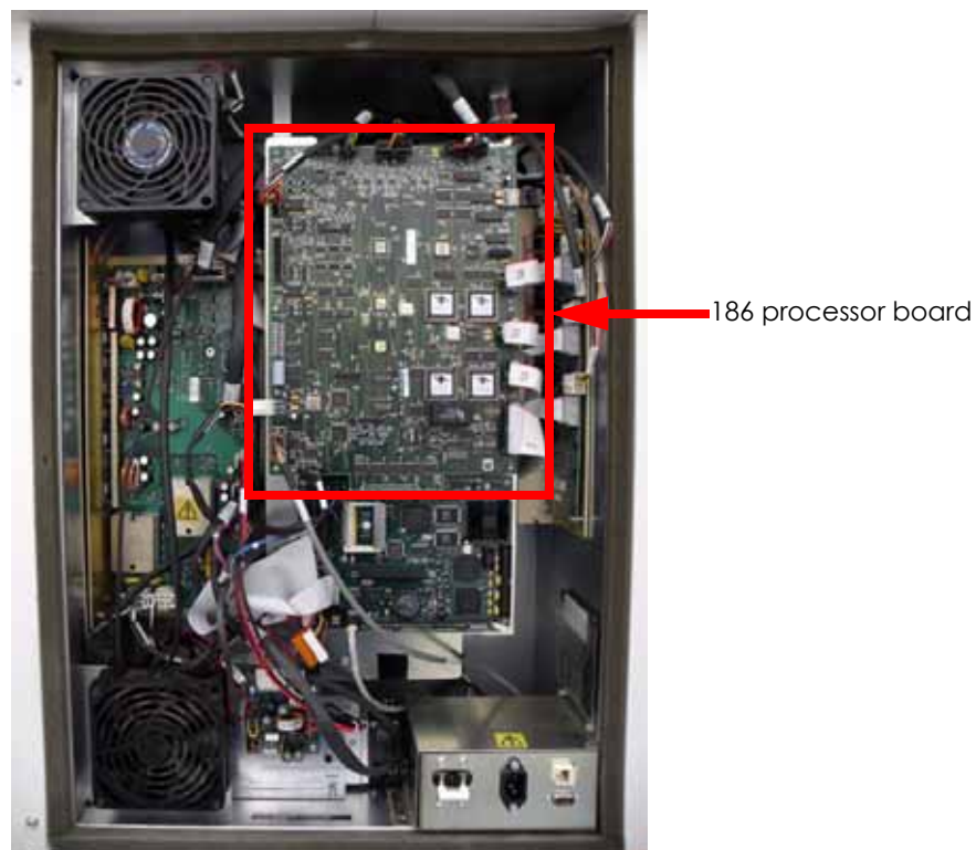
Figure 138: 186 processor board location
