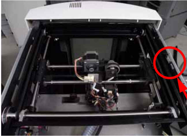
Figure 338: Y BOT sensor connector location
