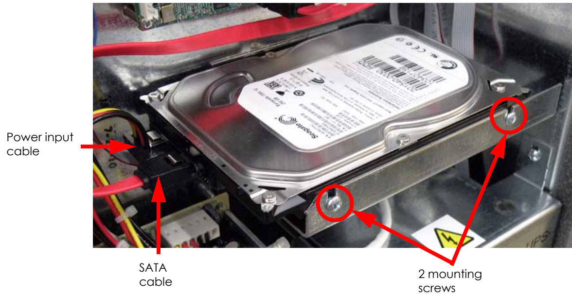
Figure 51: Hard drive connector locations
