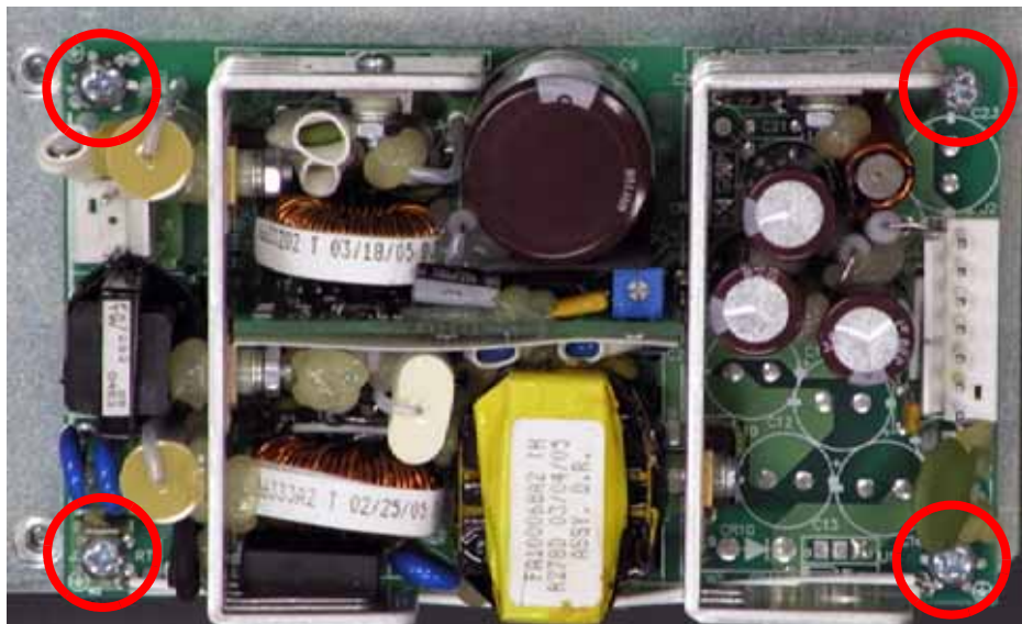
Figure 180: Dual 48 VDC power supplies mounting screw locations
