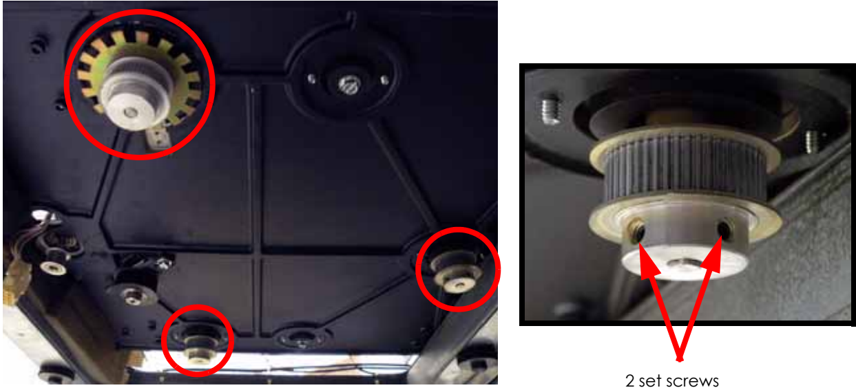
Figure 517: Lead screw pulley set screw locations
