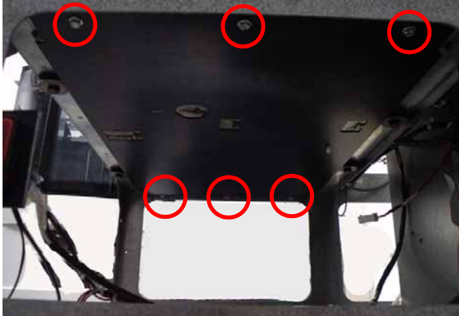
Figure 487: Z stage base plate mounting screw locations
