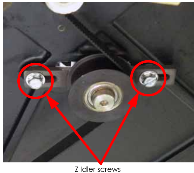
Figure 490: Z motor belt tension idler pulley screw locations
