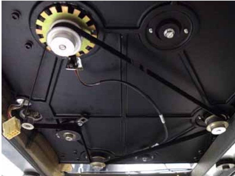
Figure 533: Z motor belt installation
