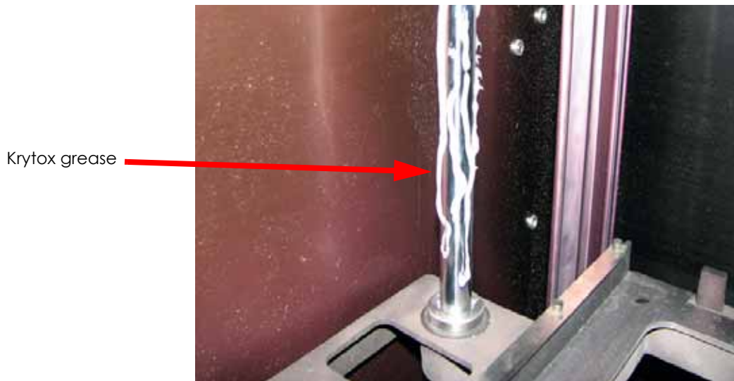
Figure 528: Apply krytox to guide rods
