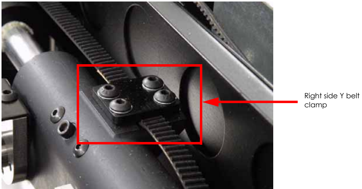
Figure 379: Right side Y belt clamp mounting screw locations
