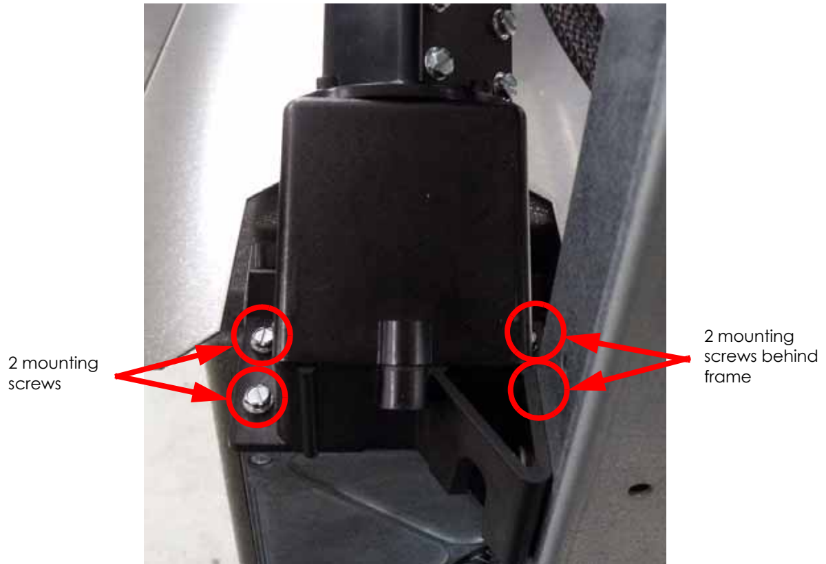
Figure 213: Hose collar mounting screw locations
