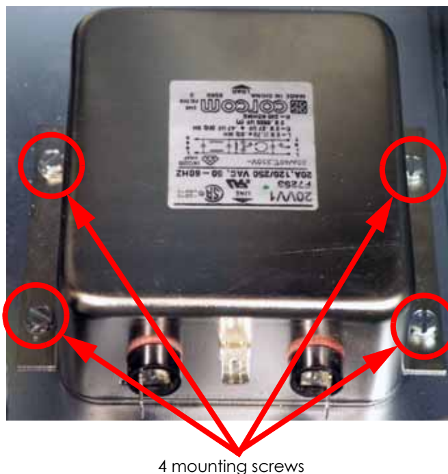
Figure 200: Line filter mounting screw locations
