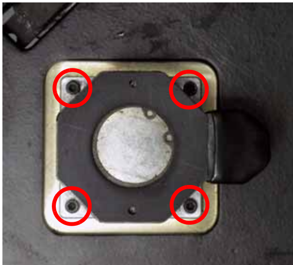
Figure 503: Z motor mounting screw locations
