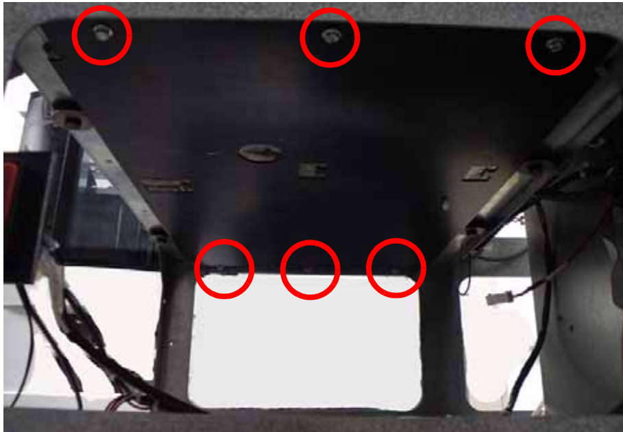
Figure 499: Z stage base plate mounting screw locations
