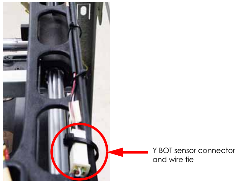
Figure 291: Wire tie and Y BOT connector locations
