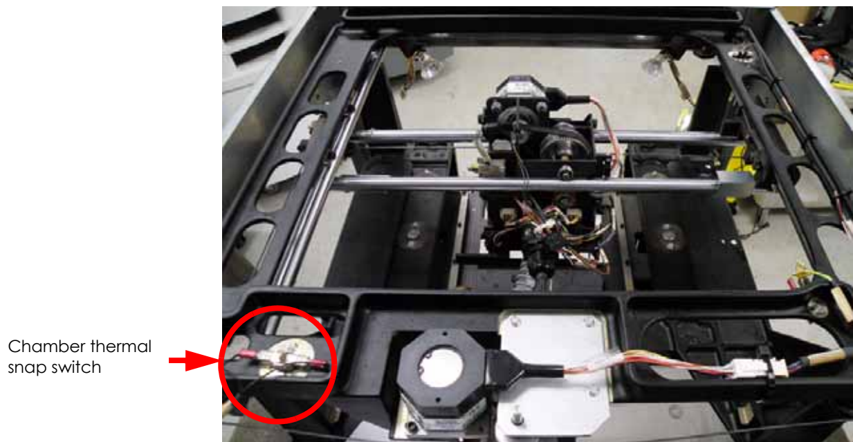
Figure 265: Chamber thermal snap switch location
