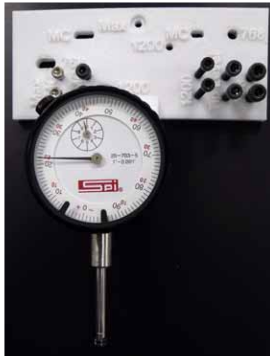
Figure 436: Dial indicator installation
