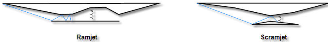
Figure 2.2: Ramjet and scramjet geometry
