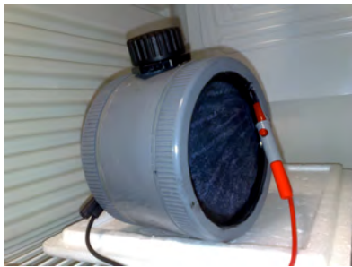
Fig. 2: Picture of 1-liter laboratory MFC
