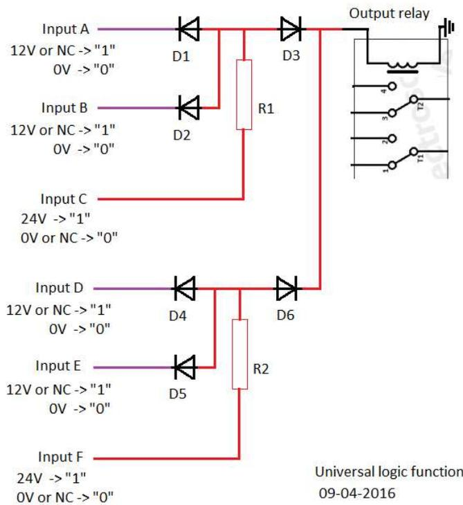
The AND function can be combined with an OR function. The circuit above shows two 3-input AND gates, the outputs of the AND gates are inputs to a 2-input OR gate (built with D3 and D6). It gives the following logic function:
