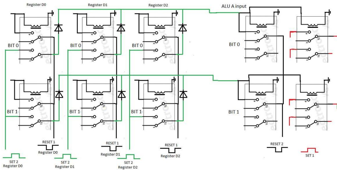
This picture has 3 data registers (for each register, only two bits are shown). The relays at the right side represent the A input of an ALU (also two bits shown, ALU function not shown).
