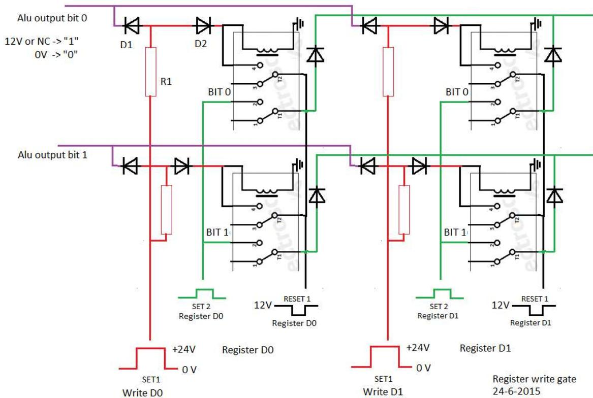
The output of the ALU is connected to several registers. We need a method to write this output to a certain register without affecting the contents of the other registers.
