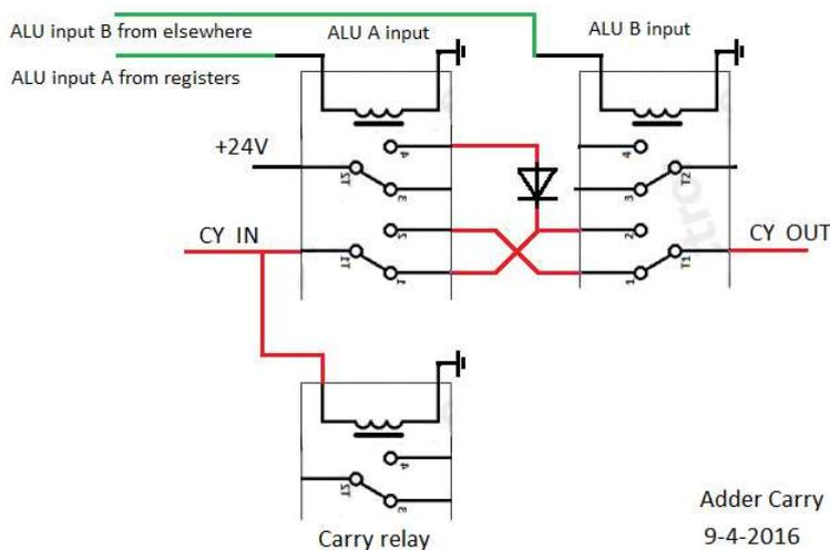
The carry is defined as active "1" if it is connected to 24V. A "0" is 0V or not connected (NC).
