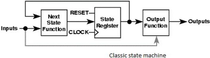
What does this state machine do ? It is characterized by the number of states that can be stored in the state register, and by the "Next State Function". If it is an 8 bit register, the state machine has 256 states. If we forget the inputs for a moment, the "Next State Function" takes the current state as input and gives the next state as an output. When the state register gets its clock signal, the state machine "goes" to this next state.
