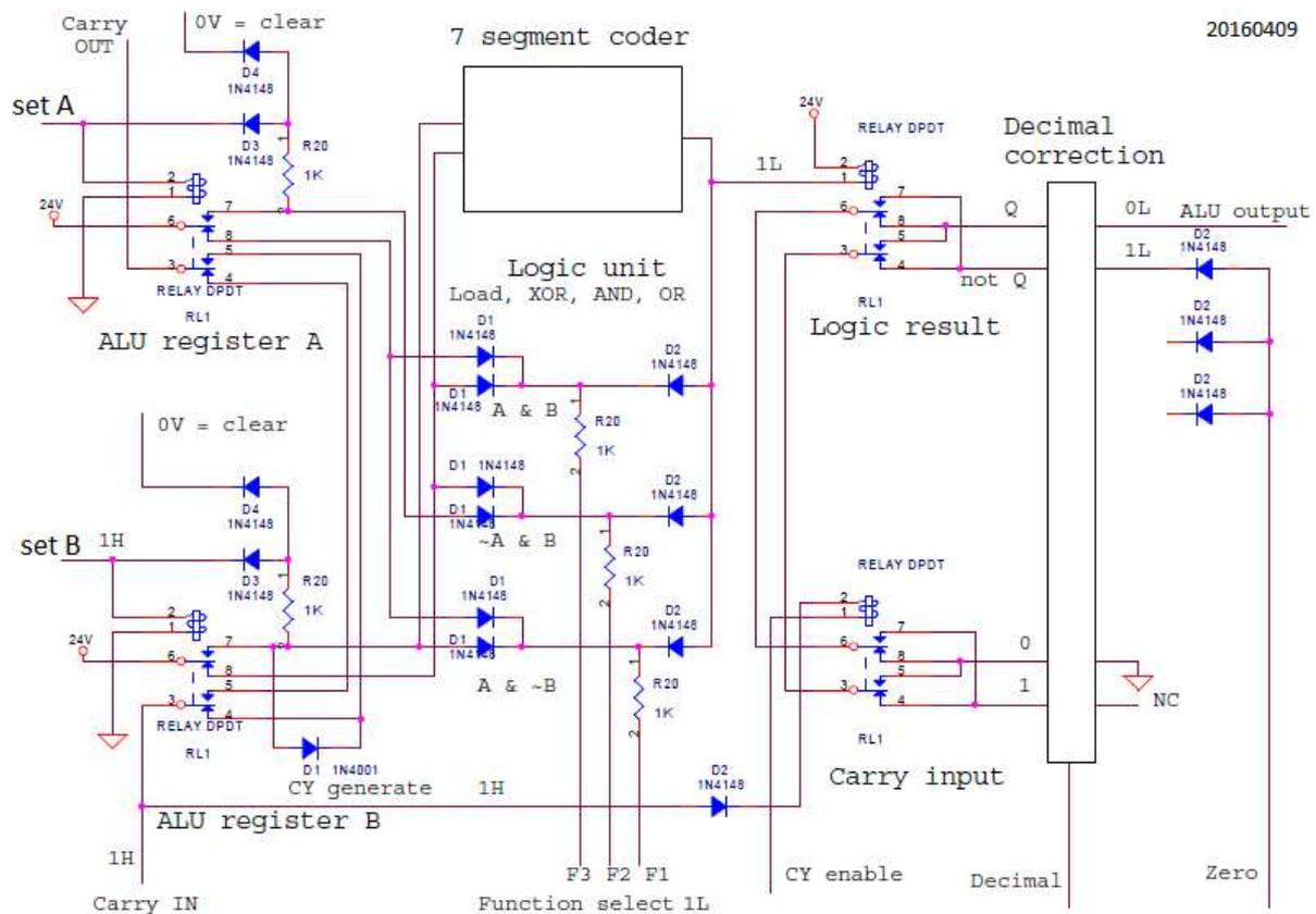
In the schematic, codes are used: 0L means logic "0" is connect to low voltage level (pulldown to ground), 1L means logic "1" is pulldown to ground, 1H means logic "1" is connect to high voltage (pull up to 12V or 24V).
