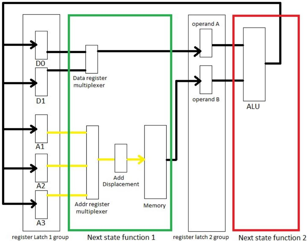
This diagram shows the most important parts of the CPU. It has the following functionality:
