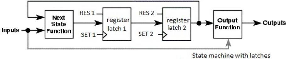
A single relay can act as a latch. The latches must be driven with a correct sequence of set and reset signals:
