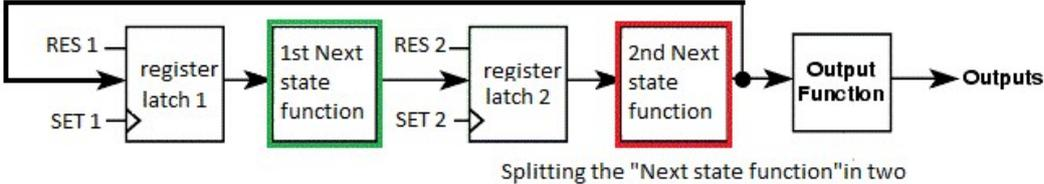
*The input has been left out of the drawing because it is not essential. The both function halves are marked green and red. Note that both register latches are not restricted to 8 bits, they can contain as many bits as you want.*
