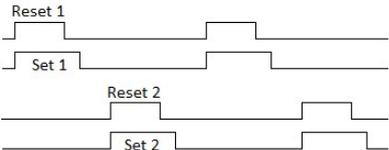
The Reset will set the latch to 0. The Set will set it to 1 if the input data (in the diagram the line with the arrow) is also 1. The effect is that after the Reset and Set signals, the latch has the same logic state as the input data.
