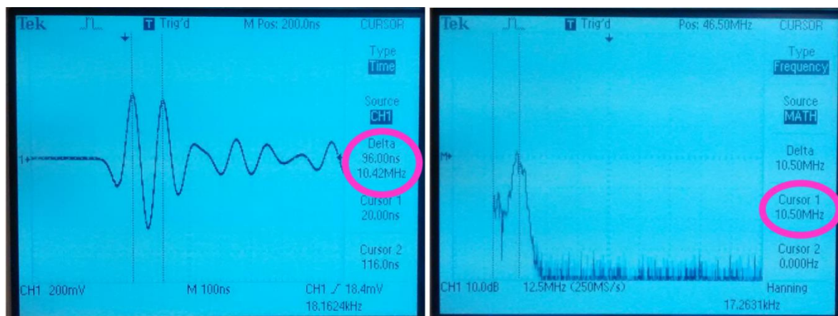
Figure 12. 16V Noise – Original – Time and Frequency Domains
