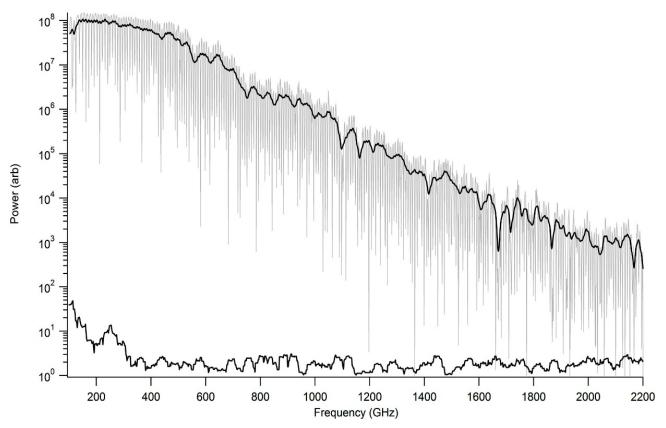
A single scan of laboratory air at 1 ATM with a PB7220-2000-T - THz Spectrometer (1 sec time constant, 1 GHz resolution) compared to the noise floor (blocked THz beam). A twenty point smoothing was applied to remove the fringe pattern for the black traces.
