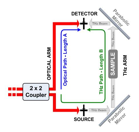
$$\begin{split} \left|L_{A}-L_{B}\right| &= \partial L \\ I_{out} \propto 1 + \cos(k \cdot \partial L) \\ k &= \frac{2\pi \upsilon}{c} n_{e\!f\!f} \\ \text{Combined sample,} \\ \text{photomixer, antenna} \\ \text{and system path} \\ \text{dispersion term} \end{split}$$
