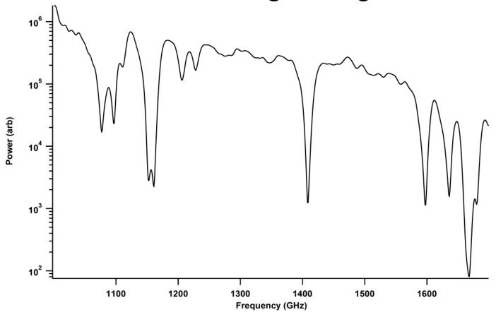
Air at 1 ATM with water vapor transitions present. An average of 10 scans. No smoothing was performed because head spacing was adjusted to remove interference fringes from the region of interest.
