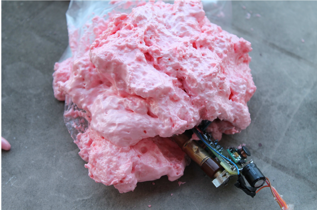
Polyurethane foam enclosing the Geiger module
