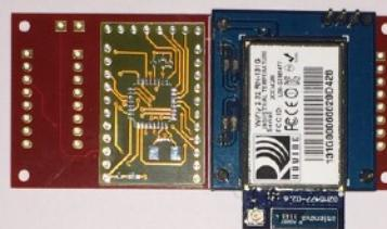
Here you can see the RN131G module soldered to a support board and placed over the backbone PCB.
