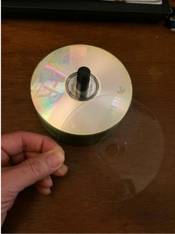
If you don't have this, you can use 1/16" clear acrylic or similar (easiest to cut) and cut a 4 1/2" square. Lay an old CD or DVD on top and use a magic marker to outline it, including the center hole. Use a scratching compass or tool to etch the circle and snap off the 4 corners.
