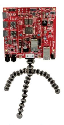
Figure 2: Avnet MicroZed Embedded Vision Kit
