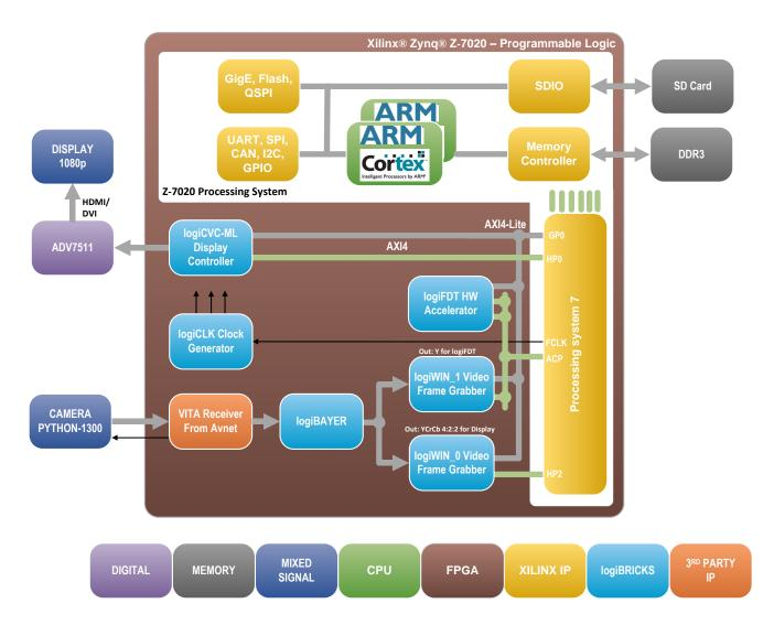
Figure 25: logiREF-FACE-TRACK-EVK Reference SoC Block Diagram
