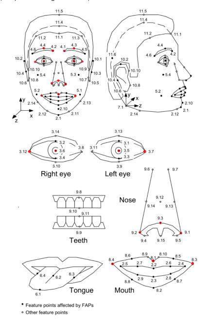
Figure 33: MPEG-4 FAB Standard Defined Facial Feature Points
