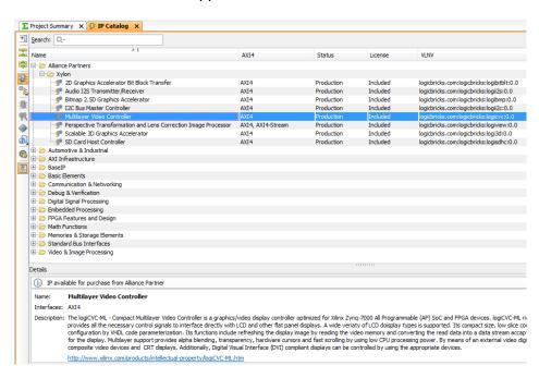
Figure 3: logicBRICKS IP Cores in the Vivado IP Catalog
