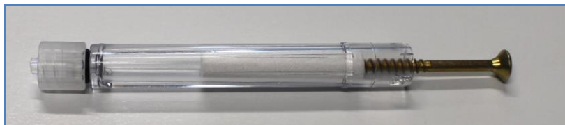
Removal of the saliva filter, using a normal screw to grab the filter
