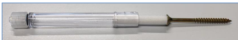
Inserting a new filter (pushing it back into the hygienic stick)
