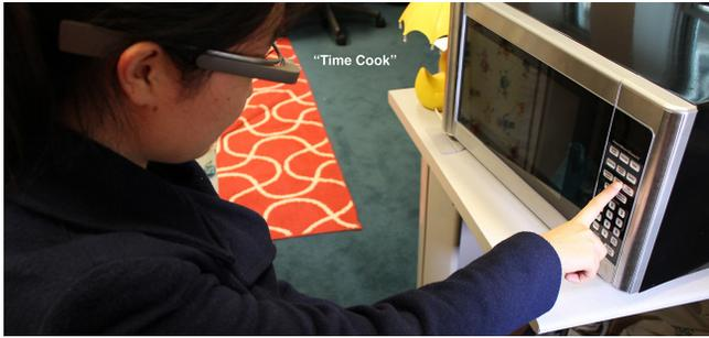
**Figure 14.** We migrated VizLens to run on Google Glass, which has the advantage of leaving the user’s hand free, easier to keep image framing stable, and naturally indicating the field of interest.
