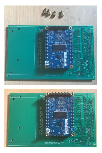
Once the four spacers have been reinstalled, the screws can be tightened.
