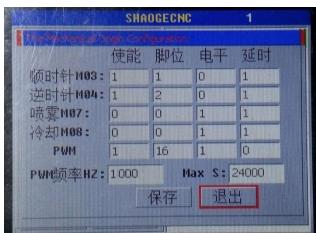
Forward connection OUT1, reverse connection OUT2, level 0 refers to the port level is low effect. PWM frequency setting 1000HZ, maximum spindle speed of 24,000 rpm.
