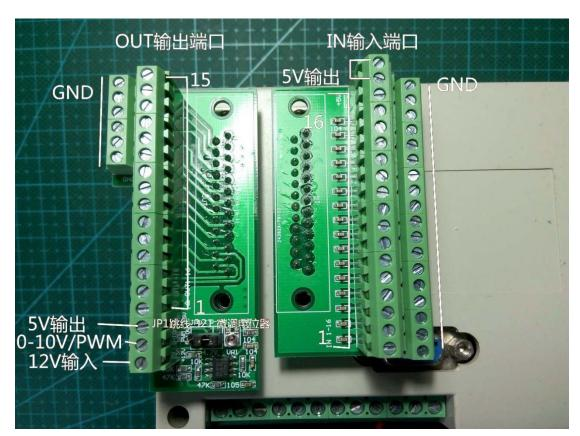
5V 输出: Controller internal 5V output, when using the total current must not exceed  $500 mA_{\circ}$
