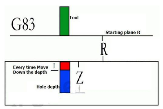
Case: (coordinates (20.0), (20.20), (0.20), (0,0) four drill holes 5mm in depth, the two safety plane, G0X0Y0Z5
