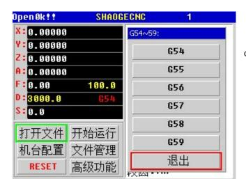
Panel shortcut key G "Workpiece coordinate system operator"
