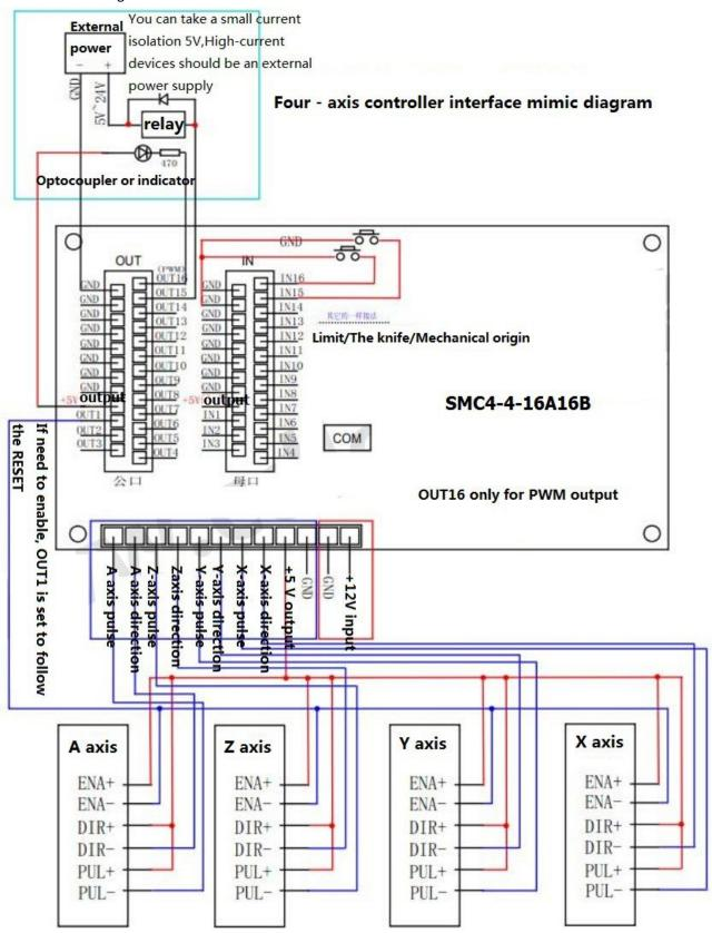
Power required to stabilize the direct pressure 12V, current should be greater than 1A, this controller is that the operating current 300MA-800MA
