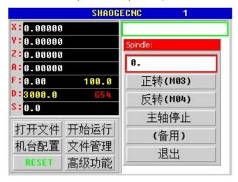
Input box to fill in the number of revolutions, the maximum value of this parameter can be set in the host settings.
