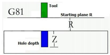
Case: (coordinates (20.0), (20.20), (0.20), (0,0) four drill holes 5mm in depth, the two safety plane, a speed of 200)
