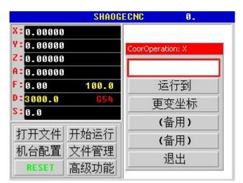
"运行到到" The corresponding axis directly run the specified coordinates.
