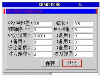
Manual Calculations or other calculation because of accuracy issues, so that the arc center is inconsistent with the values given at the moment, there is a fault-tolerant, the system will be based on the given parameters, recalculate the optimal center coordinate
