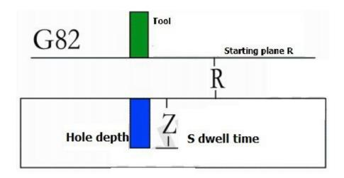
Case: (coordinates (20.0), (20.20), (0.20), (0,0) four drill holes 5mm in depth, the two safety plane, and one second stay at the hole bottom, a speed of 200)
