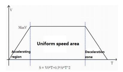
Acceleration values: the ability to be finalized in accordance with the motor, based on not fall out step, take 70% of maximum speed values , leaving 30% margin to the motor (characteristics of stepper motor).
