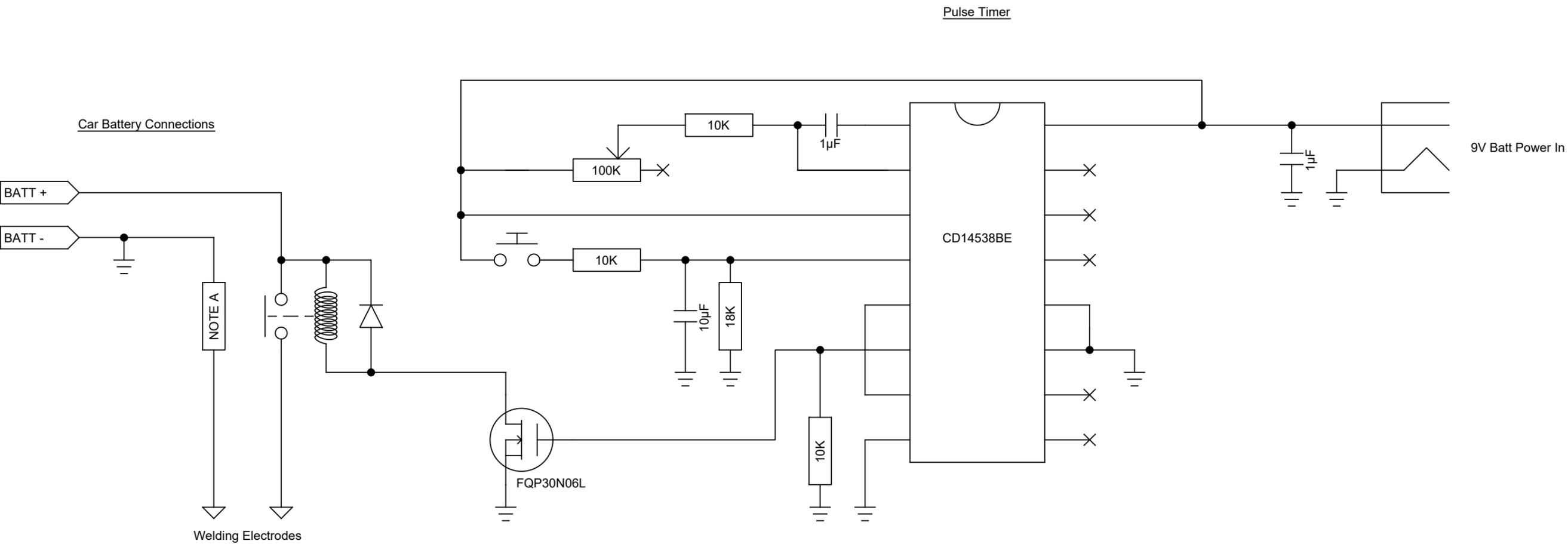
NOTE A: Current limiting resister formed of aprox 50mm long 1.6mm OD steel rod immersed in water for cooling
