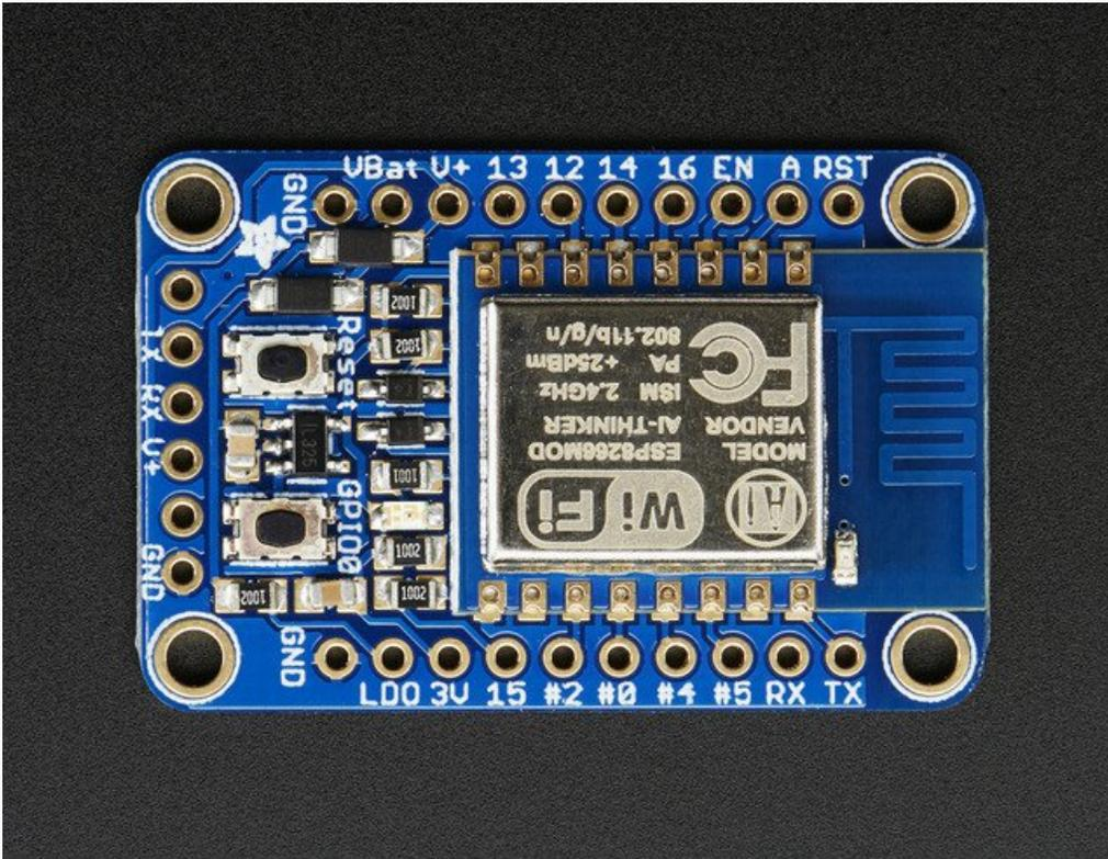
The HUZDAH ESP8266 breakout is what we designed to make working with this chip super easy and a lot of fun. We took a certified module with an onboard antenna, and plenty of pins, and soldered it onto our designed breakout PCBs. We added in:
