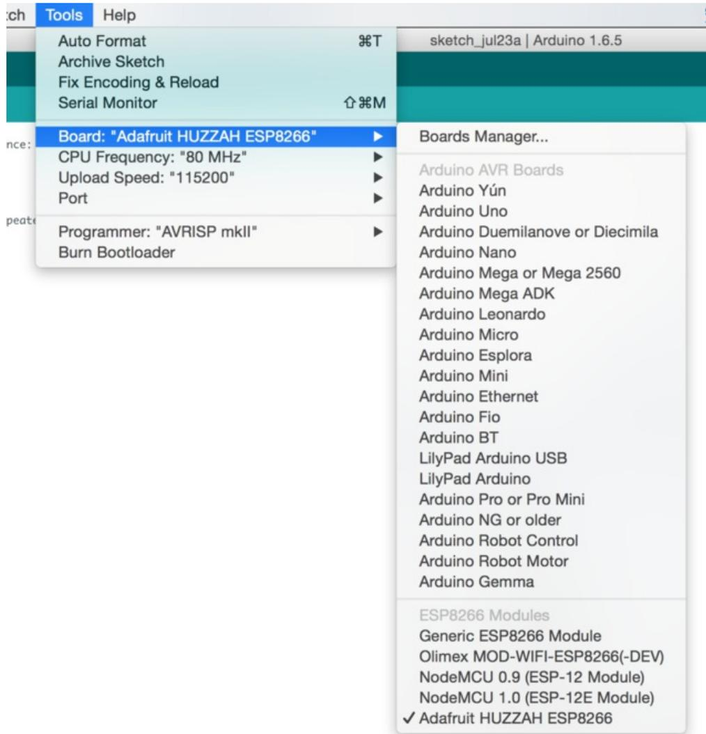
80 MHz as the CPU frequency (you can try 160 MHz overclock later)
