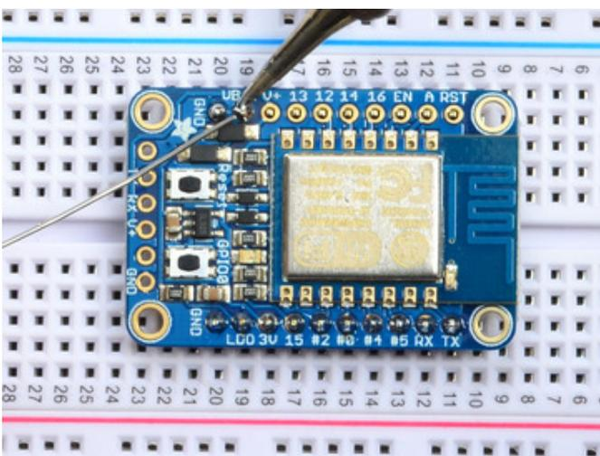
Flip the breadboard around to solder the other strip
