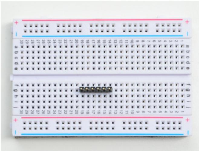
If you're planning on programming with an FTDI or console cable, it's handy to have 6 pins soldered on the end for plugging in.
