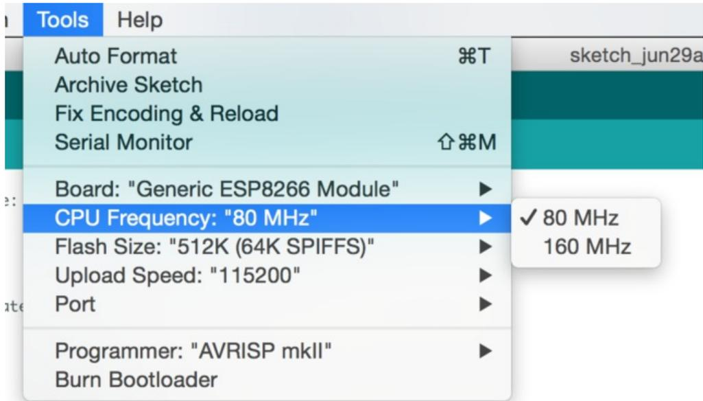
115200 baud upload speed is a good place to start - later on you can try higher speeds but 115200 is a good safe place to start. You can move down to lower speeds if you are having upload issues, or speed it up if your setup is stable, for faster uploads!
