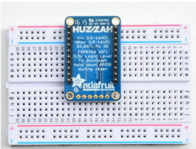
Place the breakout on the breadboard facing down
