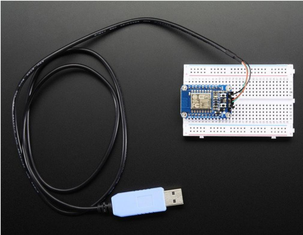
Each module comes pre-loaded with NodeMCU's Lua interpreter (NodeMCU 0.9.5 build 20150318 / Lua 5.1.4 to be specific), you can run commands, and 'save' Lua programs directly to the module's Flash using a USB-Serial converter cable.
