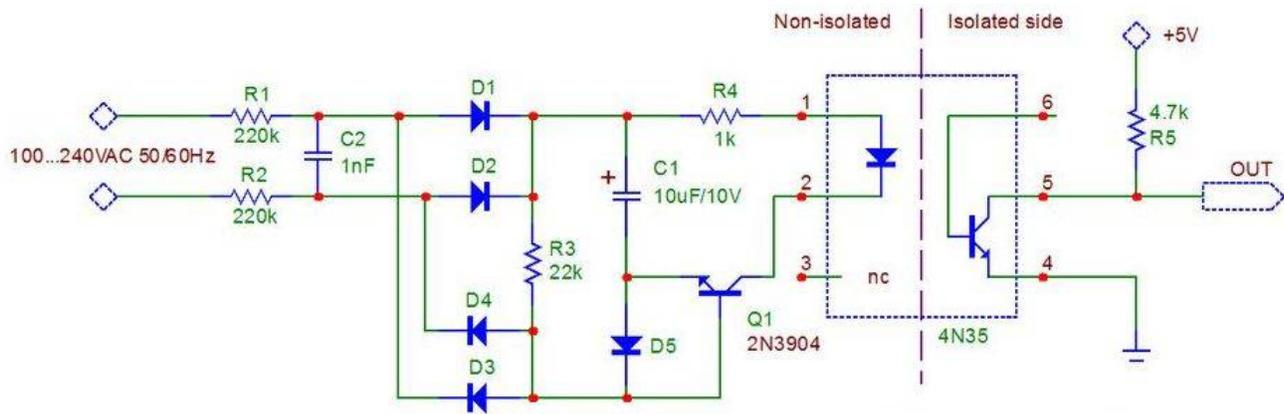
FIGURE 1. Isolated, precision zero-crossing detector schematic.
