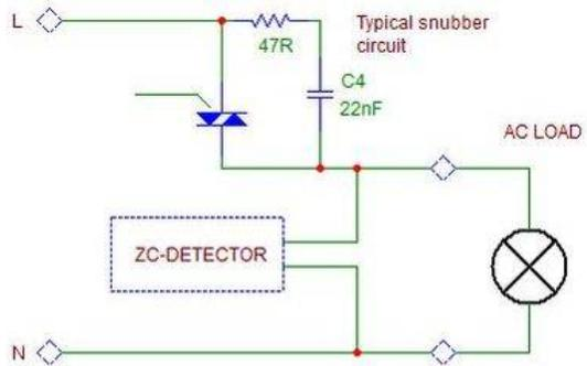
Fig. 5 - Example of load monitoring. The triac snubber produces enough of current to detect if the load is disconnected. Likewise, the ZC-detector can tell if power is delivered to a connected load.
