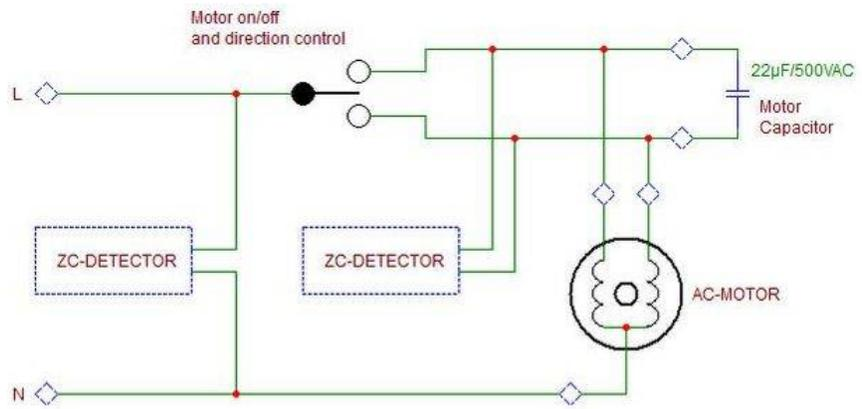
Fig. 6 - AC-motor monitoring circuit. The first ZC-detector determines the existence of the mains voltage and gives the microprocessor a reference zero crossing signal. The other ZC-circuit measures the phase difference (or its zero crossing occurrence). If the delay between the two ZC-circuits is within predetermined limits you can be sure of that the motor rotates.
