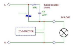
Fig. 5 - Example of load monitoring. The triac snubber produces enough of current to detect if the load is disconnected. Likevise, the ZC-detector can tell if power is deliveret to a connected load.
