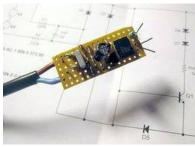
Fig. 2 - Prototype circuit built on perfboard
