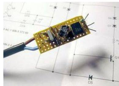
Fig. 2 - Prototype circuit built on perboard
