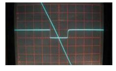
Fig. 3 - Actual scope image of a zerocrossing. Y-scale for the mains voltage is 20V/div and 5V/div for the output signal. Zero is at centerline. Time scale is 500us/div.
