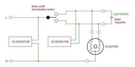
Fig. 6 - AC-motor monitoring ciruit. The first ZC-detector determines the existence of the mains voltage and gives the microprocessor a reference zero crossing signal. The other ZC-circuit measures the phase difference (or it's zero crossing occurence). If the delay between the two ZC-circuits is within predetermined limits you can be sue of that the motor rotates.
