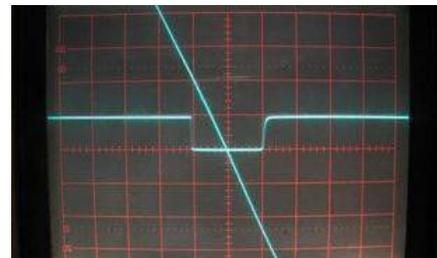
Fig. 3 - Actual scope image of a zero-crossing. Y-scale for the mains voltage is 20V/div and 5V/div for the output signal. Zero is at centerline. Time scale is 500us/div.
