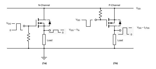
FIGURE 1. Comparing the Performance Between N-Channel and P-Channel Grounded-Load Switching
