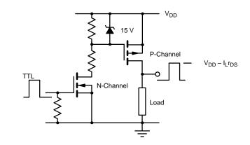
FIGURE 3. Using An N-Channel Level-Shifter Simplifies Driving From Logic
