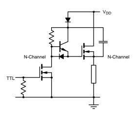
FIGURE 2. Bootstrapping for N-Channel Grounded-Load Switching
