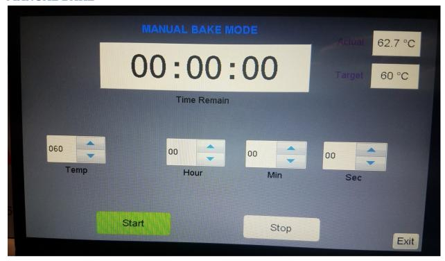
The manual bake menu allows you to set a desired target temperature (initially sets the Temp to the 'pre-heat' temp in the config.ini). You can choose the number of hours, minutes, and seconds that you would like the manual bake to run. The start button is initially green, once pressed, it will become disabled, and the Stop button will become RED, and it will be enabled.
