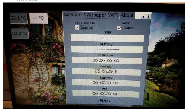
The WiFi tab allows you the configure all of the parameters of your wifi connection, including using DHCP, or specifying a manual IP address.
