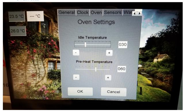
The oven tab allows you to configure the oven 'idle temperature', which is the temperature that the 'cool' button on the main page will attempt to hold the oven at if pressed. The 'pre-heat' temperature is the temperature that the 'pre-heat' button on the main page will heat the oven to, when pressed.
