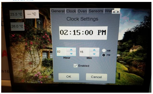
The clock tab allows you to configure the time of day, HOURS, MINS, and AM/PM. Currently there is no seconds settings, as you can get close enough with hours/mins. Possibily in a future release this can be added if necessary.
