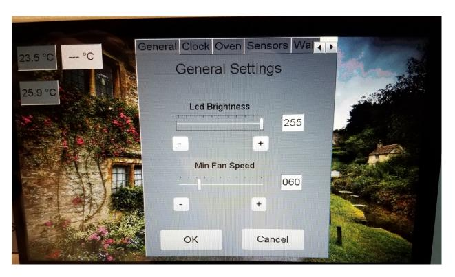
The general tab allows you to configure the LCD brightness, from 10 to 255 (255 = max brightness). The slider will not allow you to go down to below 10, since below 10 the screen is completely dark and you cannot see anything.
