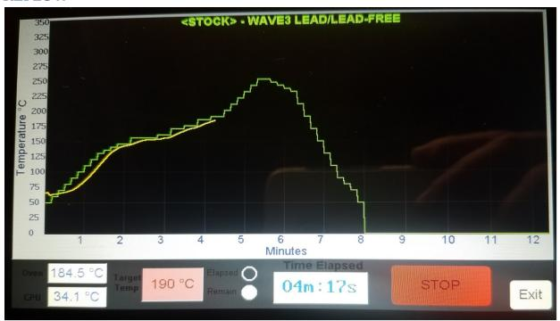
The reflow GUI is where you actually run a reflow profile. It will display the last profile that you chose in the 'profile' menu. The target profile is displayed in **GREEN**, and the running profile will update every second, and is displayed in **YELLOW**.
