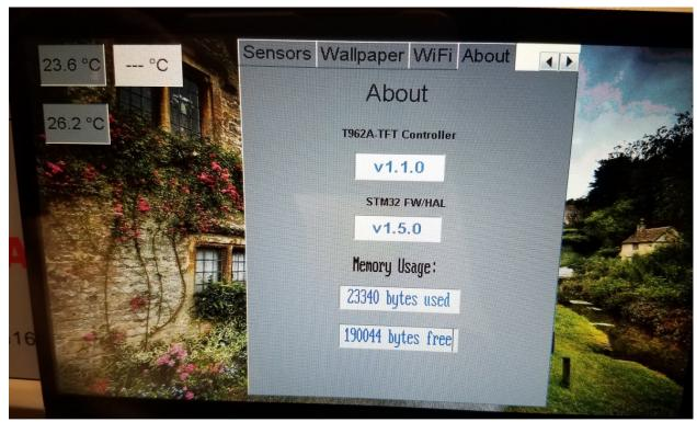
The about tab is an informational window only. It allows you to see your current controller software version, the STM32 HAL version that it's running on, and how much memory the STemWin GUI software is using, and how much is free.
