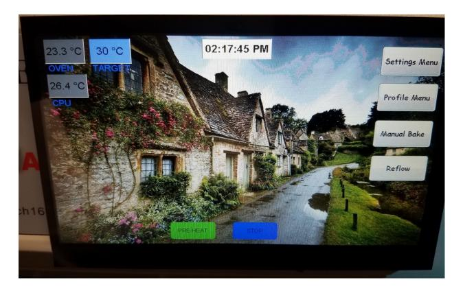
The top left corner is temperature status for the OVEN, CPU (controller board itself, ie what we've known as CJ temp), and TARGET temp, which is the desired temp if 'pre-heat' or 'cool' button was pressed. If in idle, ie no pre-heat or cool pressed, the 'TARGET' box will display '---'.
