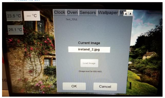
The wallpaper tab allows you to change the background wallpaper of the main menu. The 'current image' box displays the name of the current image that is the background. Clicking on the 'Load Image' button will bring up a file dialog box, showing all ".JPG" files found in the "images\" folder on the microsd card. (This folder already exists in the microsd files included with this software).
