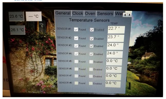
The sensors tab will show you all sensors that have been detected, ie via the 'found' checkbox. The 'found' checkbox is a read-only checkbox, the software will check the box if it finds a sensor at that address. The TEMP box will display the current temperature for each sensor it finds. The 'Enabled' checkbox can be enabled/disabled by touching the checkbox.
