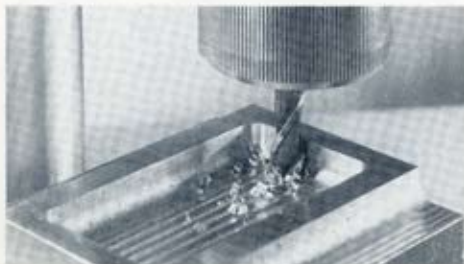
WITH BALL END MILLS you can mill filleted recesses, rounded grooves or small die cavities.
