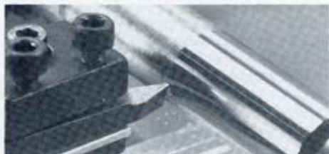
FINISH CUTS taken at high spindle speed with a round-nose tool leave a very smooth finish.
