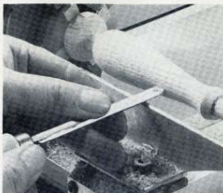
A MACHINEX 5 OWNER can make many accessories for the machine himself. Example: a tool rest for woodturning chisels cut from angle steel and mounted on the worktable with T-bolts.
