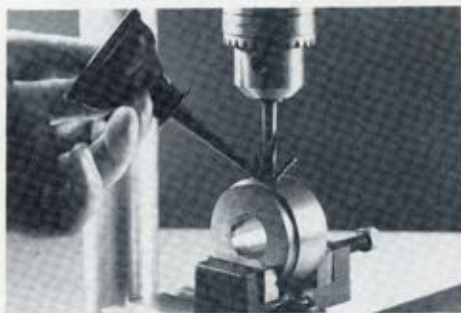
WORK TO BE DRILLED in the drill press can be mounted on the worktable in the machine vise.
