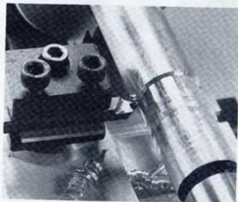
ROUGHING CUTS taken at slow spindle speed remove metal rapidly but leave a rough finish.
