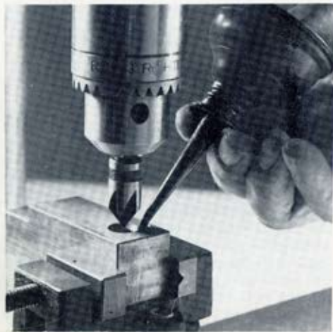
USE CUTTING OIL and work at slow spindle speed when countersinking or counterboring steel.
