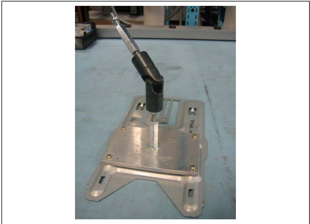
Figure 2-32. Test Fixture Attached to SRM for the Pull Test
