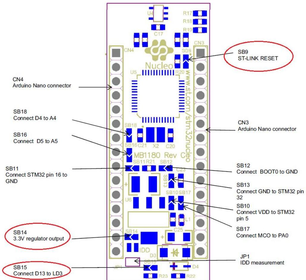
Warning, the removal of these soldered jumpers is a quite difficult operation. It is easy to make big mistakes.
