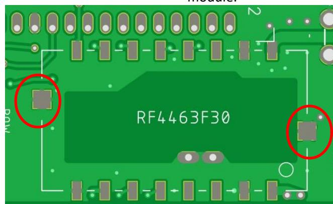
For all RF4463 solders, you should heat the whole PCB and/or module to 80-100°C while soldering (with a standard soldering iron), for example via a cooking plate.
