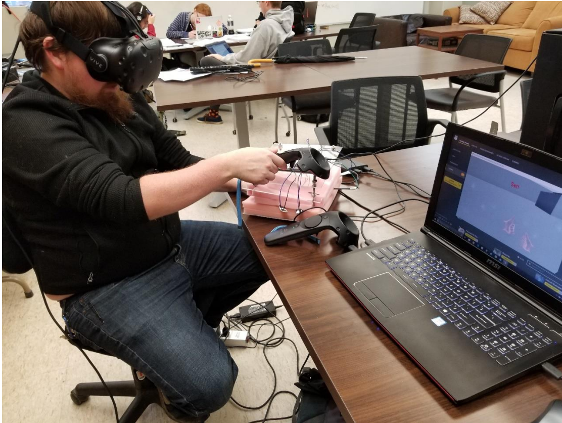
Figure 5. A user making a thumbs up with his left hand and controlling the entire hand's location in space with the motion controller in his right hand.
