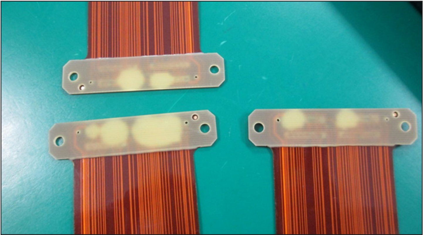
Image of stiffener delamination due to lack of pre-bake prior to assembly.
