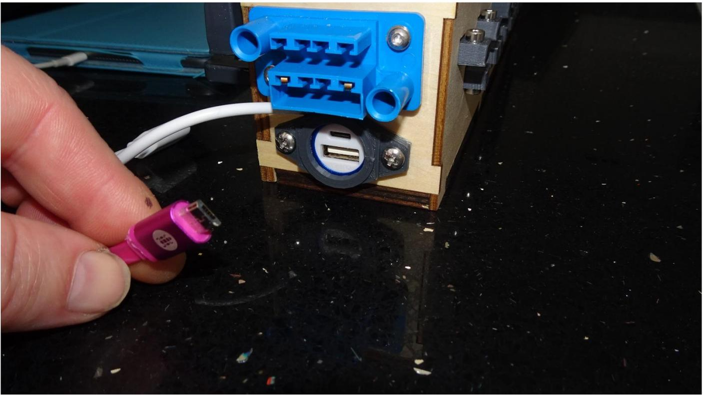
**Charge the battery by inserting a phone charger into the smaller socket (micro-USB). End of the battery holder module will glow green when charged.**
