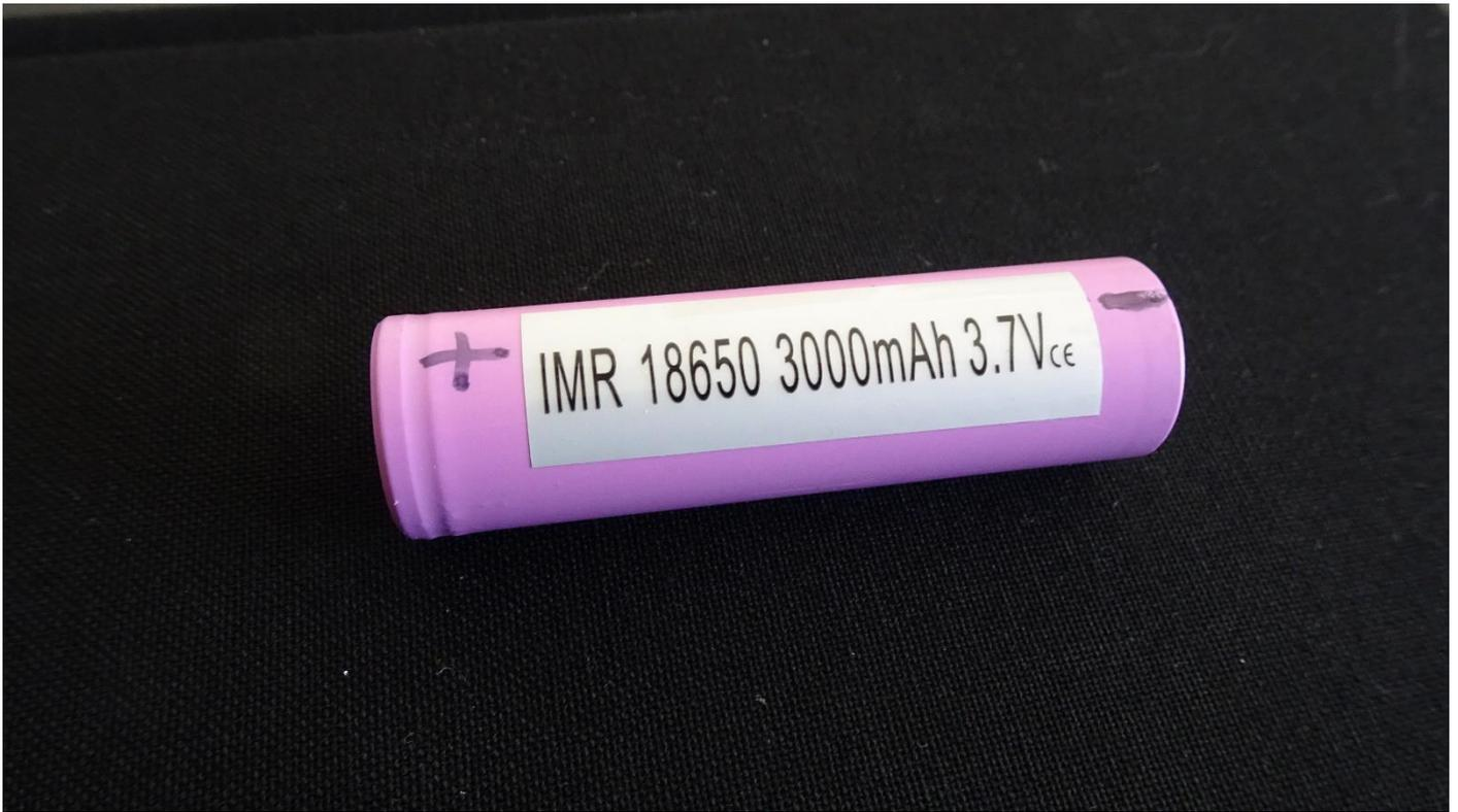
**NOTE:** You must use the type of 18650 that does NOT have a bulge on the +ve terminal. Both ends must be flat but both types are out there so be sure to buy the correct one. The +ve terminal has a ridge next to it that runs around the battery case as in the photo above.
