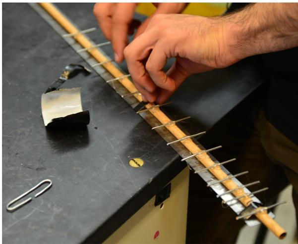
Fig. 5: Yagi antenna
