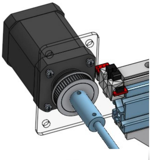
Then add the second bracket with the 4 bolts and the spacer between the brackets. Finally add the 5 mm screws to the T – Nuts in the Y axis.
