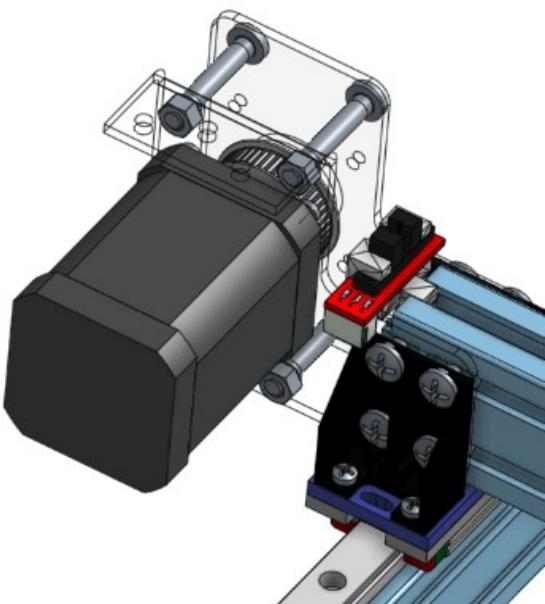
However, this time you need to add the black 3D printed bracket that holds the X axis to the slider assembly. Here is a picture with the bracket in place.
