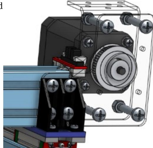
Here it is with the cable chain mounted on it.
