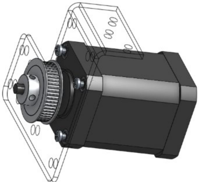
Now just like the idlers, you need to put the 4 M5 x 6 screws through the bracket and into the 5 mm T nuts. The T-nuts can be seen on this view.
