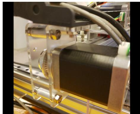
Don't forget to mount the Black 3D printed brackets on the other side of the X axis by the idler. It is the same process.
