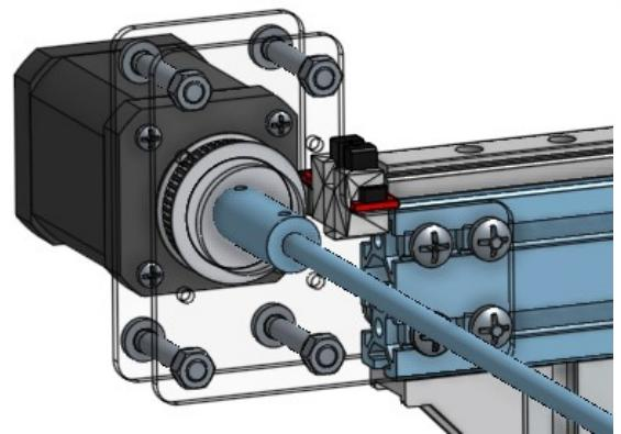
The same drill on the other side here for the slave axis. First attach the 50 tooth pulley. Then the join the *brass bracket* to the shaft. Lastly attach the 2 M5 x 6mm screws through the Brass bracket into the 2 M5 T nuts.
