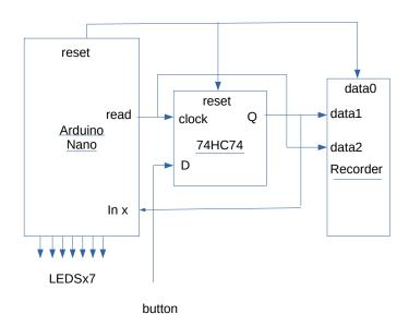
Currently the ck for the flipflop, its "q" output and the reset signal is drawn out from the Arduino. The reset signal is used for the initial synchronization.
