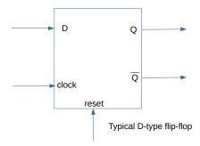
Here the idea is that one output from the nano is responsible for triggering the flip-flop and thus sample the value of the button. Connected to the 'D' pin. The observant code reader might already have noted that this takes place in the dice.ino code. Yes we need code modifications for this hack to happen since we are not doing it inside the MCU with dedicated hardware as in the first figure.
