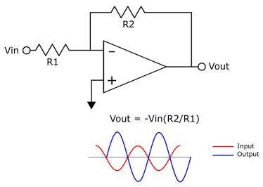
The above illustration shows the inverting op-amp configuration, and its gain formula (also called a transfer function). The incoming signal is both amplified and inverted.
