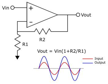
The above illustration shows the non-inverting op-amp, and its gain formula. The incoming signal is amplified, and not inverted.
