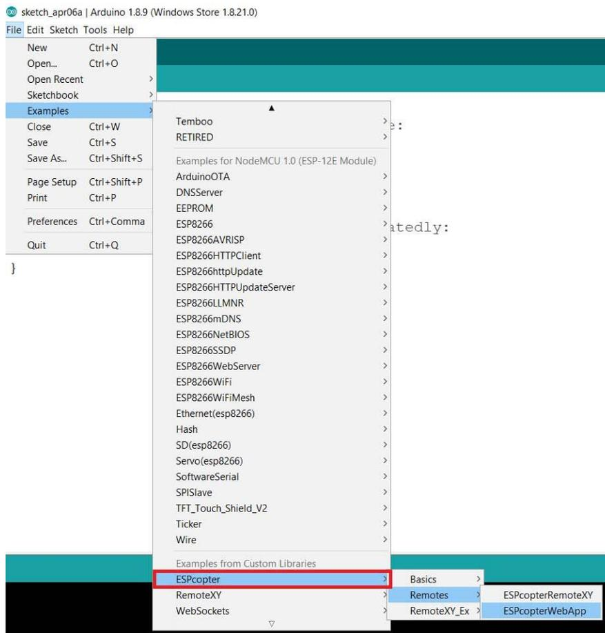
The ESPcopter will have the flight control software to make the flight stable. This ESPcopterWebApp example is a demonstration of the ESPcopter having the additional ability to act as a self-contained web server. This will get you running your ESPcopter fast because you can control it from a web page on your phone, tablet or laptop. More advanced examples (Although this is very cool) are already available from the Arduino IDE menu.
