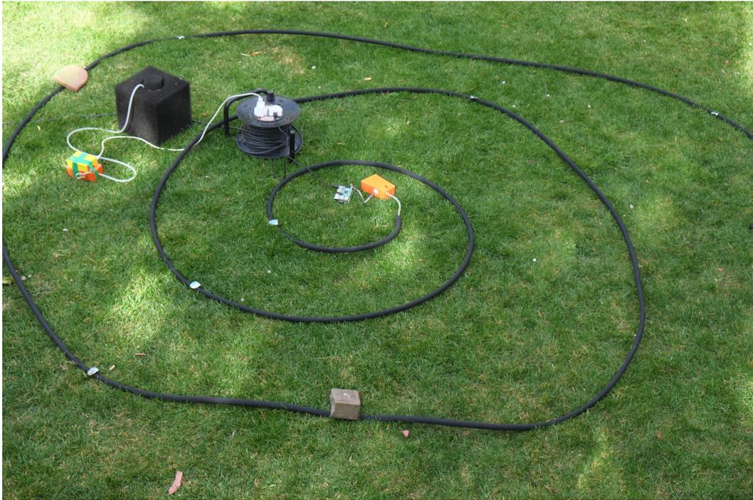
Figure 8: Pond filter tested alongside spiral hose
