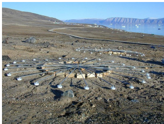
CTBTO Infrasound Array, Greenland
