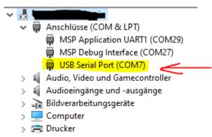
10. Go back to your target configuration and type in the desired baud rate and the COM Port:
