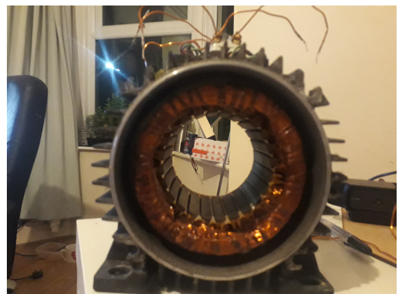
(b) Three Phase AC Induction stator for test
