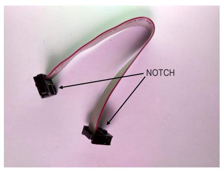
• Finally connect the RF switch and the tinker board with the FRC cable, again paying attention to the notch (we've had enough of the notch!).
