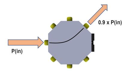
4. Average isolation between selected port and other ports = <u>26dB</u> => <u>0.002 x P(in)</u> The power level of the leaked or coupled signal on the unselected ports is as low as 0.002 times (or -26dB) the power level on the selected port.
