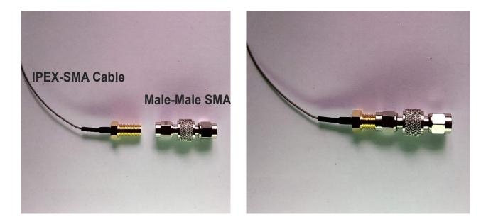
Connect the IPEX port of the IPEX-SMA cable to the IPEX port on the green RF board (not the IPEX port of the on board antenna) by lining it up carefully and pressing it down with your nails or a small hard surface like the end of toothpick till you feel a "click/snap". Check the connection by gently applying tension on the cable.
