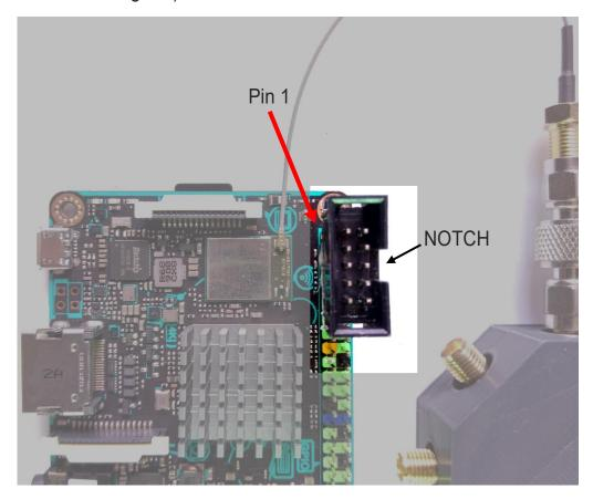
• Get 10 pin FRC cable and make sure that the notches on both ends line up on the same side.
