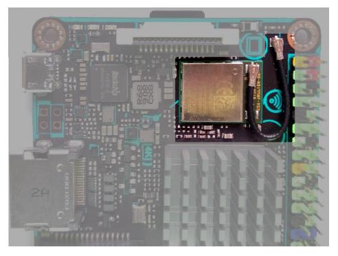
• Carefully unplug both ends using a pair of tweezers.
