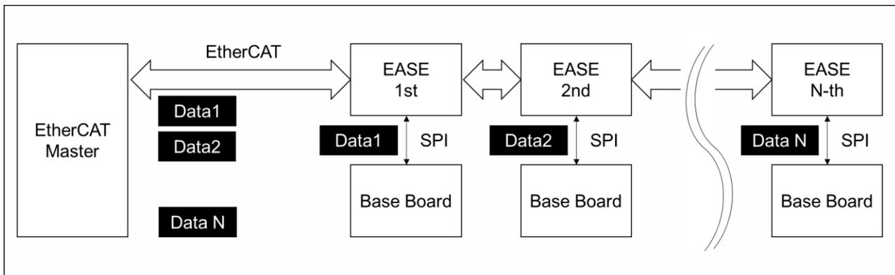
FIGURE 14. DATA FLOW BETWEEN ETHERCAT MASTER, EASE, AND BASE BOARD
