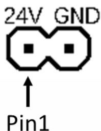
FIGURE 6. X3, 24VDC POWER SUPPLY CONNECTOR
