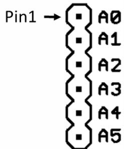
FIGURE 8. X5, ANALOG INPUT CONNECTOR
