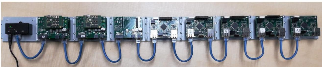
FIGURE 17 EXAMPLE OF AN DAISY CHAIN CONNECTION OF ESMACAT SLAVES FOR ETHERCAT COMMUNICATION AND POWER SUPPLY WITH POE
