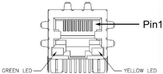
**FIGURE 5. X1/X2 ETHERCAT IN/OUT RJ45 CONNECTOR**
