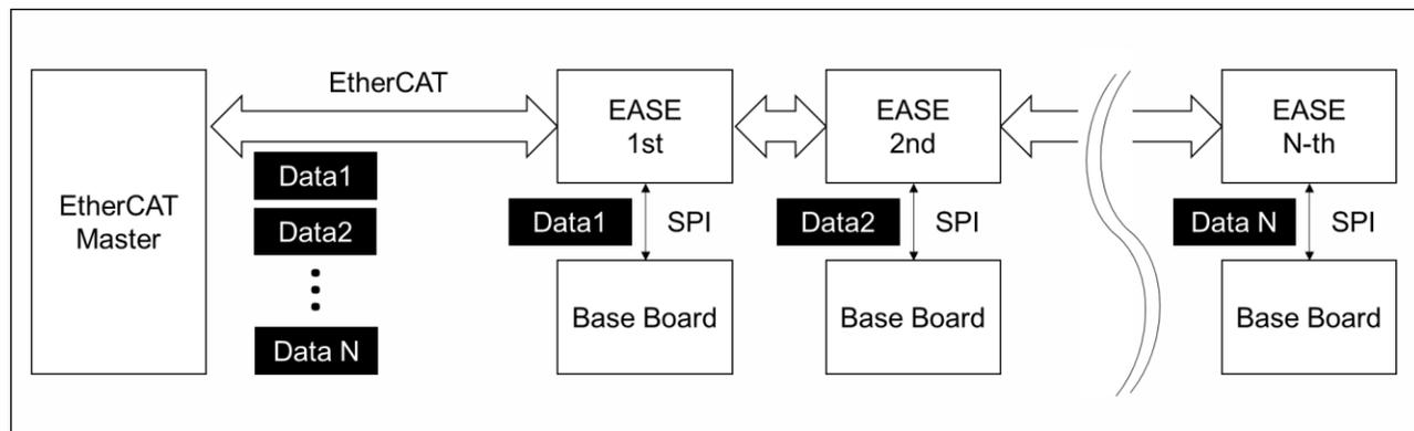
FIGURE 1. DATA FLOW BETWEEN ETHERCAT MASTER, EASE, AND BASE BOARD
