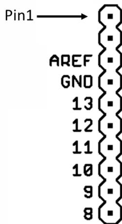
FIGURE 9. X6, COMMUNICATION CONNECTOR
