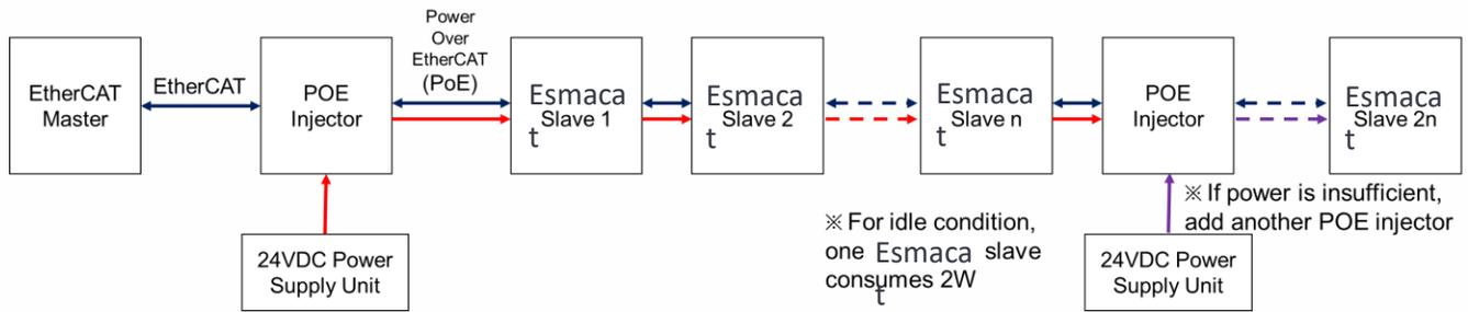
FIGURE 18 LOGIC POWER SUPPLY VIA POE
