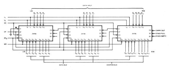
FIGURE 1. 34706 EXPANSION A 16 BY 12 PROGRAM STACK
