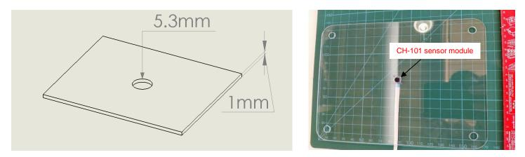
Figure 6. Recommended MOD\_CH101-03-01 module mounting
