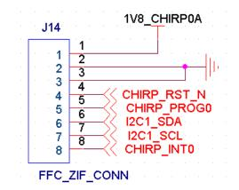
Figure 4. Flat flex cable connector motherboard side pin layout
