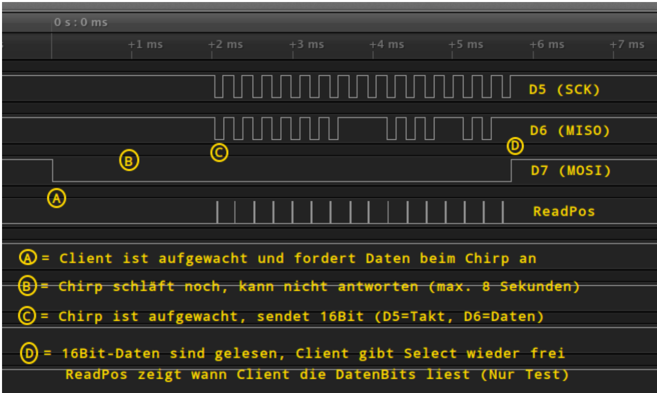
Data protocol between client and Chirp
