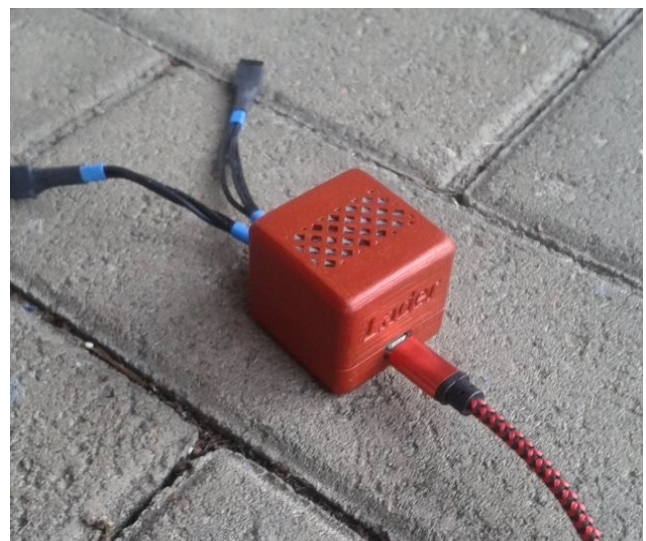
LiFePo4-USB-Charger in housing
