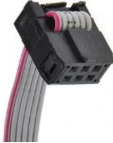
Fig.11 6 Pin Programming Connector
