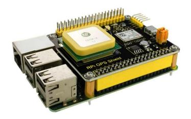
For the Raspberry Pi 3 you need to explicitly enable the serial port on the GPIO pins. The reason for this is a change with the Pi 3 to use the hardware serial port for Bluetooth and instead use a slightly different software's serial port for the GPIO pins.
