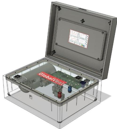
Figure 1: BostonVent CAD Model
