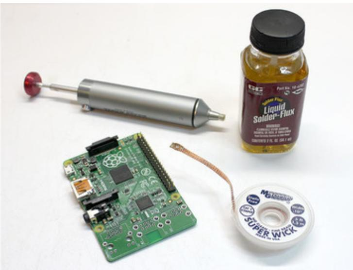
Solder wick is heated under the tip of the soldering iron and rubbed across the areas to clean...this soaks up solder like a paper towel! **Do this on both sides of the board.** Applying liquid soldering flux first (either the brush-on or pen applicator type) makes this process a little smoother and cleaner.
