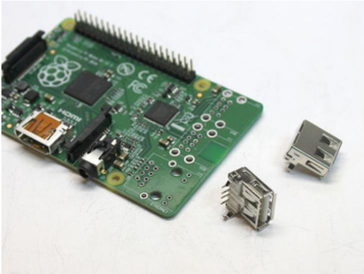
You can install one or two replacement USB ports, depending on your needs. Unlike the old stacked ports, these are single-height, so two is the maximum.
