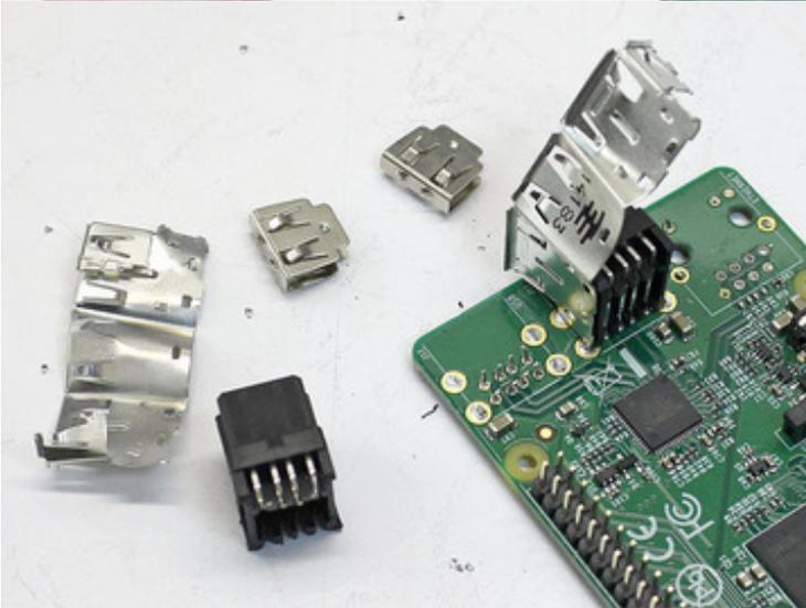
The USB ports similarly required a lot of grappling. Rather than trying to desolder the pins and pry the housing off the board, the housing was dismantled and the pins were clipped from the component side, and the schrapnel will be cleaned up later.
