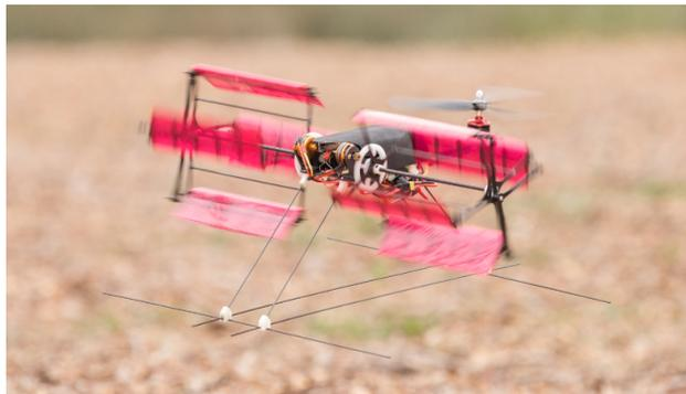
Figure 38: Dual cyclocopter platform.
