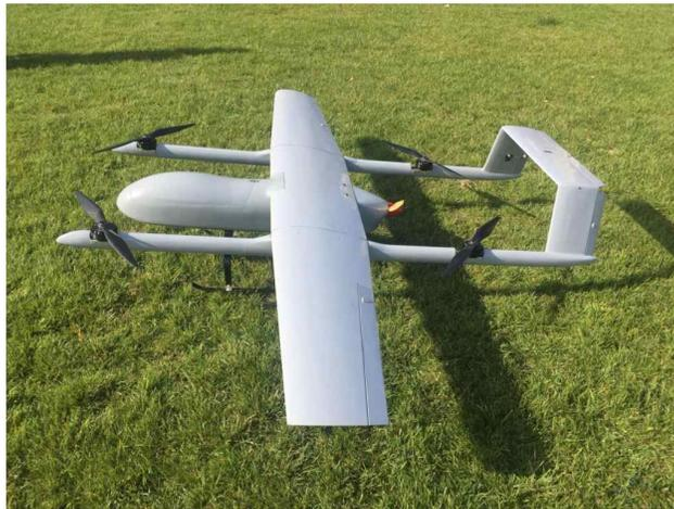
Figure 35: Simple VTOL configuration that acts like a quadrotor in hover and a conventional fixed wing aircraft in forward flight.
