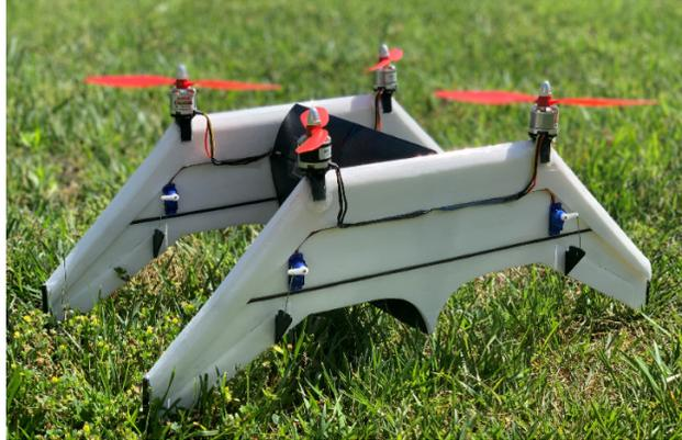
Figure 37: Quadrotor Biplane VTOL platform.
