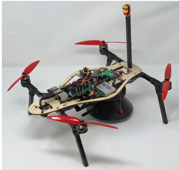
Figure 36: Simple quadrotor platform.
