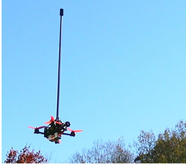
Figure 42: Racing drone balancing an inverted pendulum.
