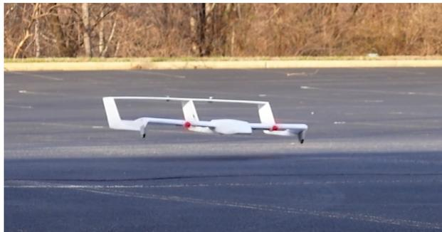
Figure 43: Fixed wing ground effect vehicle.
