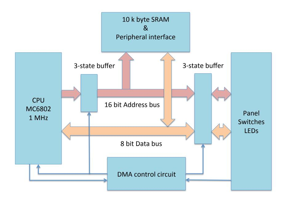
Fig 1 PERSEUS-3 Hardware block diagram
