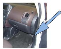
The hood release is under the instrument panel beside the front passenger's door.
