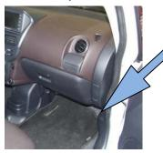
The hood release is under the instrument panel beside the **front passenger's** door.
