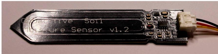
**Figure 3.** A “capacitive” soil moisture sensor. The grazing light image shows the coplanar concentric capacitor of the sensor.
